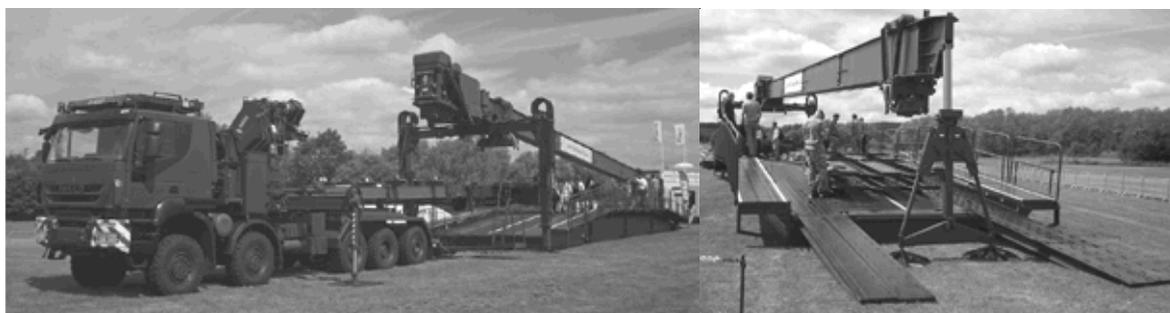
**Fig. 6. Span of the "Swiss" version of DSB with sidewalk and handrails with a launch vehicle on a IVECO Trakker 10×8 chassis**
