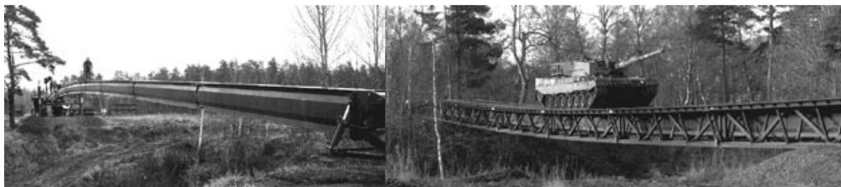
**Fig. 7. View of the launch beam extended to the opposite bank and the complete FB 48 bridge set over an obstacle (launch beam between lattice girders) [18]**
