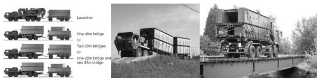
**Fig. 4. Schematic drawing of the M18 DSB set, CBT Oshkosh M1077 transport vehicle with M1076 trailer and IVECO 8×8 transport vehicle [16]**
