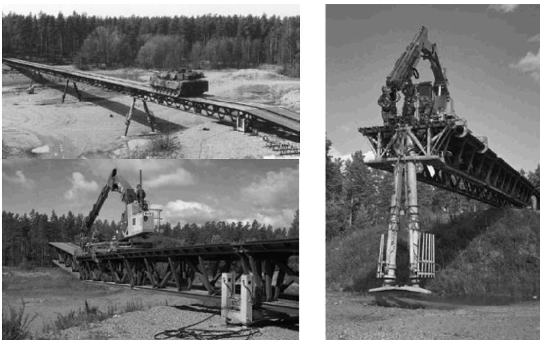
**Fig. 9. The FB 200 bridge over an obstacle and launching of the span segments and of the support by means of a special launcher [18]**
