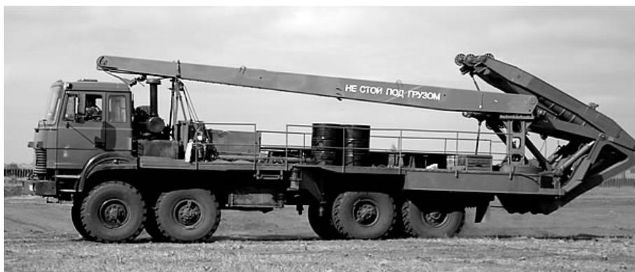
**Fig. 10. Launching vehicle (MCM) of the MMK bridge [21]**
