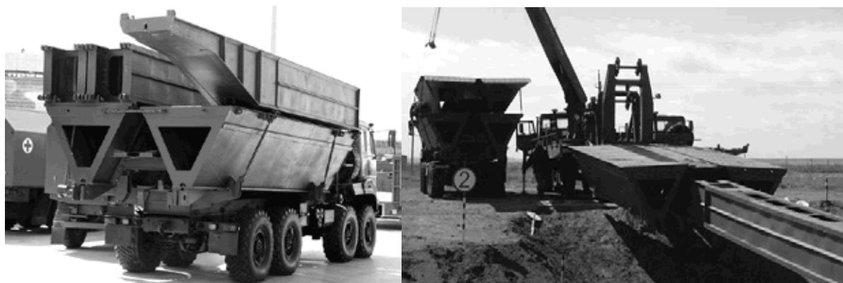
**Fig. 11. View of the segments of the bridge and of the launching beam in the transport position and assembly of the MMK span segments on the launching beam [21]**
