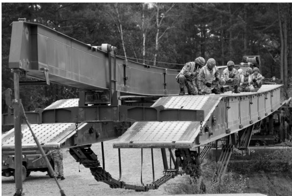
**Fig. 12. GSB construction with strengthening system under the span [26]**
