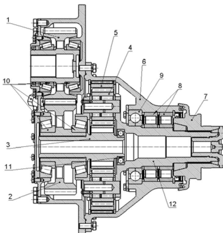
**Fig. 3 Proposed design of the final drive**
