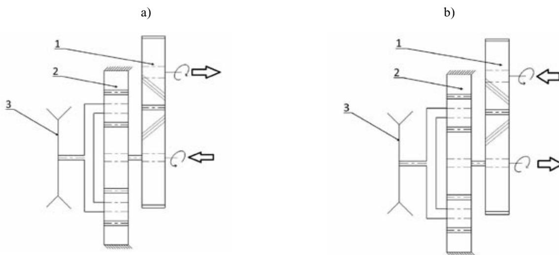
**Fig. 4. Directions of axial force action in the final drive**
