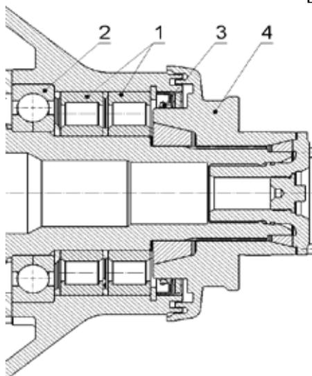
**Fig. 5. Carrier bearing on final drive output**
