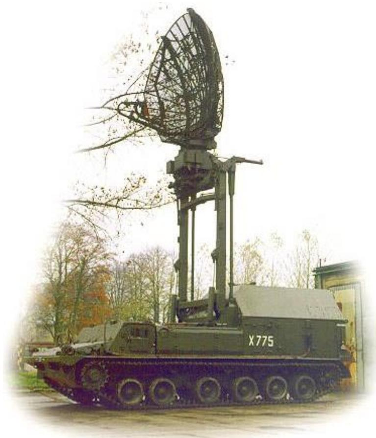
**Fig. 2. NUR-21M radar station on SPG-1M tracked chassis**
