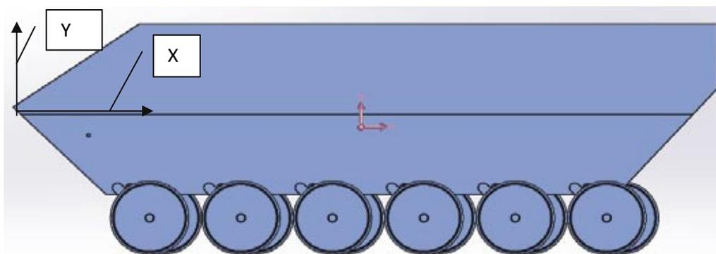
**Fig. 1. Computational model of the hull (Z axis perpendicular to the drawing plane)**
