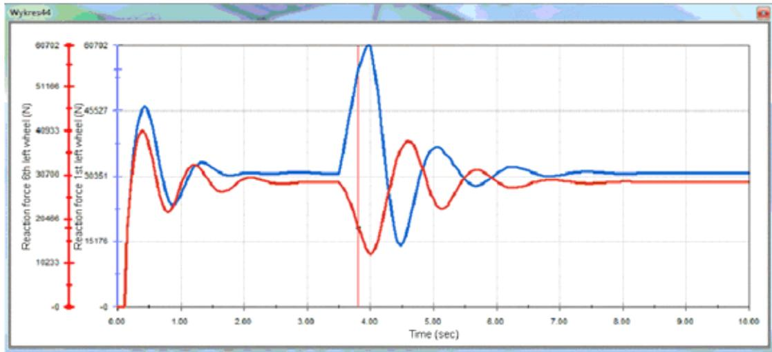
Fig. 7. Wheel loads on the left side (1st wheel - blue) and accelerations of the hull (6th wheel - red)
