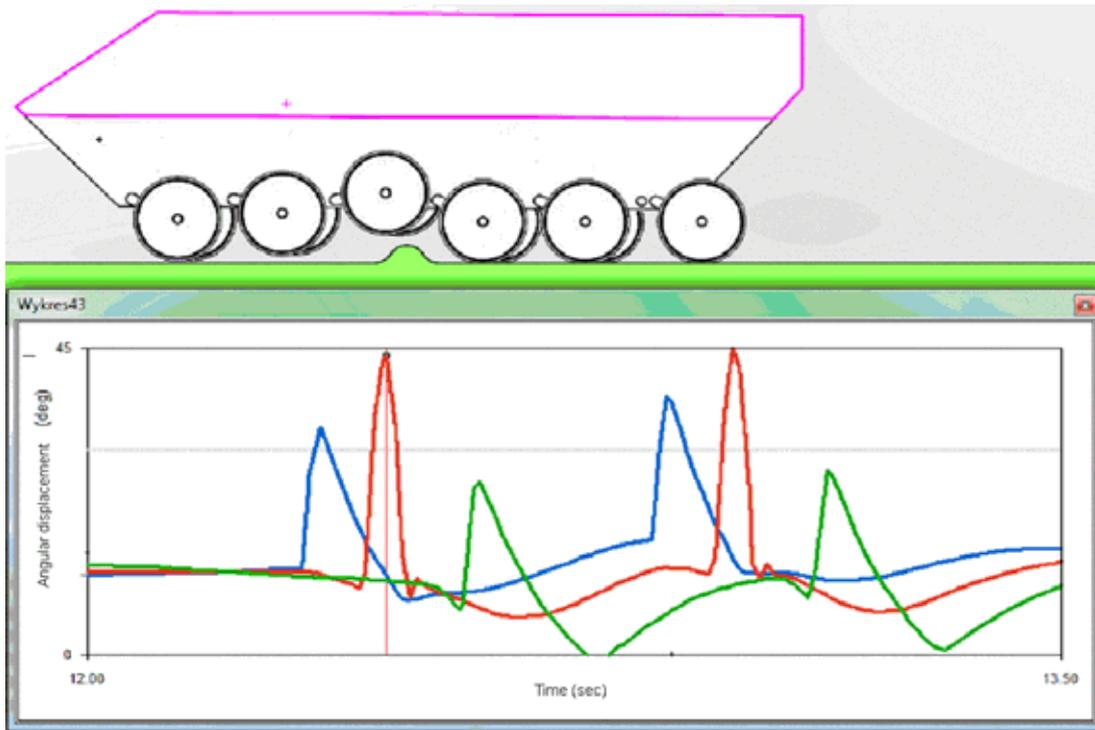
**Fig. 14. Angular displacements of the suspension arms on the left side (1st wheel - blue, 3rd wheel - red, 6th wheel - green)**
