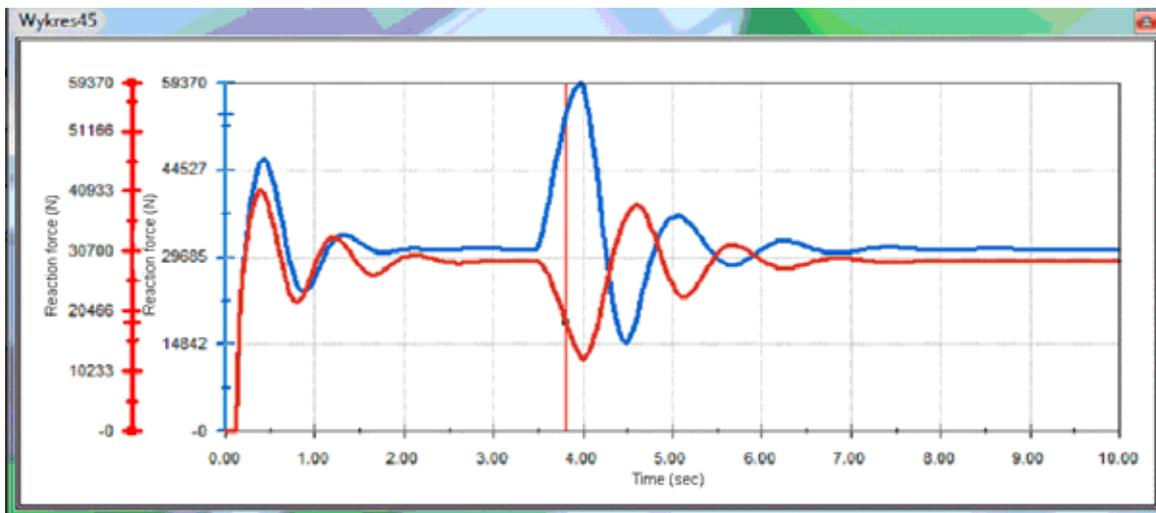
Fig. 8. Wheel loads on the right side (1st wheel - blue) and accelerations of the hull (6th wheel - red)
