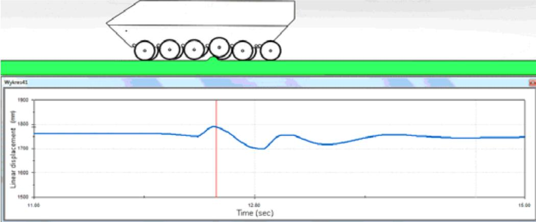
**Fig. 12. Graph of the displacement of the front edge of the hull (vehicle shown when the 4th wheel is over the bump)**
