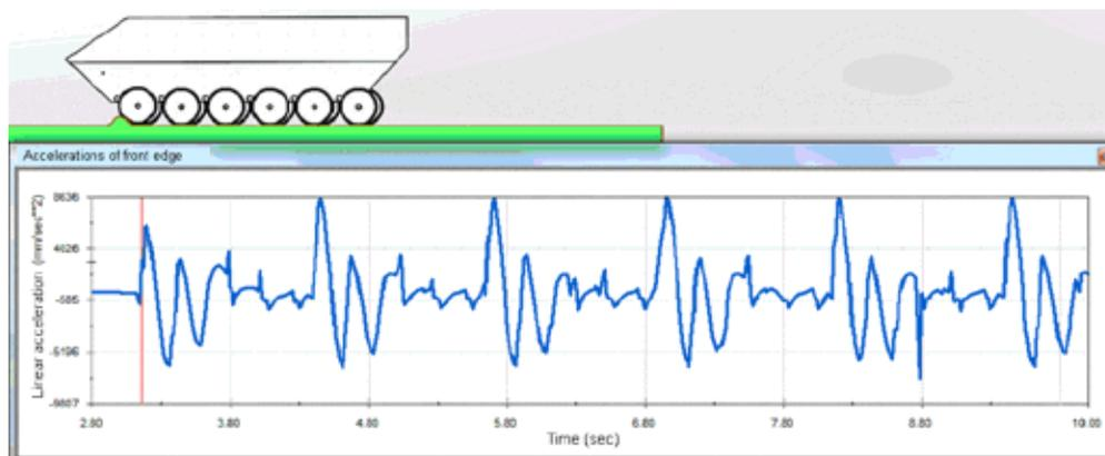
**Fig. 16. Graph of the acceleration of the front edge of the hull (vehicle shown just before reaching the obstacle)**
