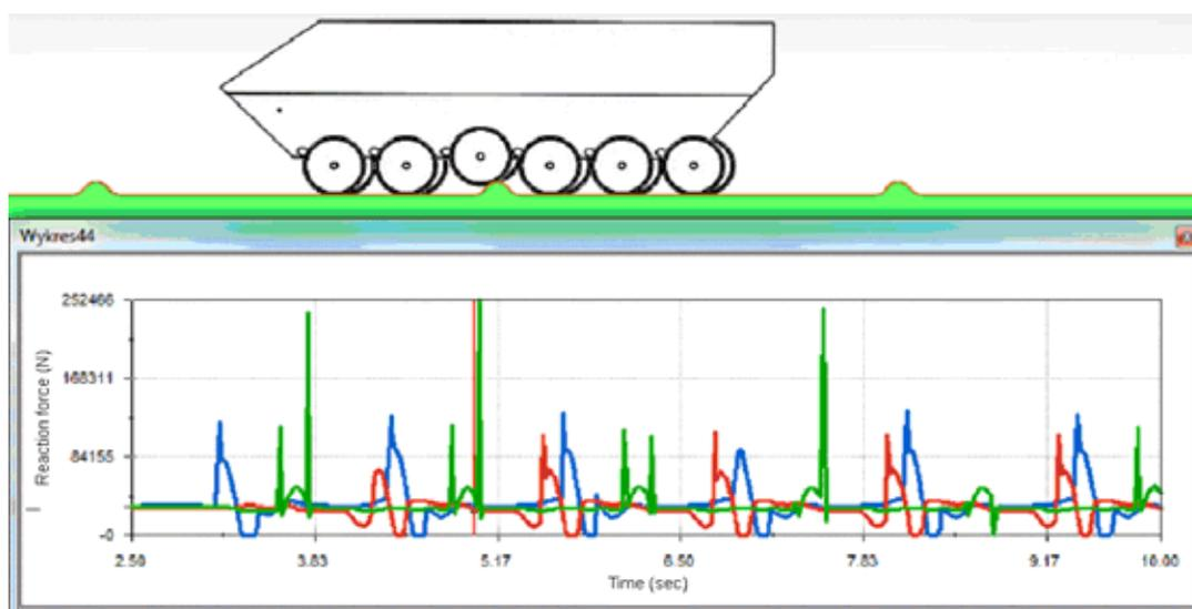
**Fig. 18. Wheel loads on the left side (1st wheel - blue, 3rd wheel - green, 6th wheel - red)**
