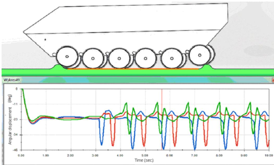
**Fig. 19. Angular displacements of the suspension arms on the left side (1st wheel - blue, 3rd wheel - red, 6th wheel - green)**
