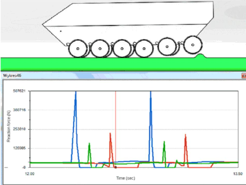
**Fig. 13. Wheel loads on the left side of the hull (1st wheel - blue, 3rd wheel - green, 6th wheel - red)**
