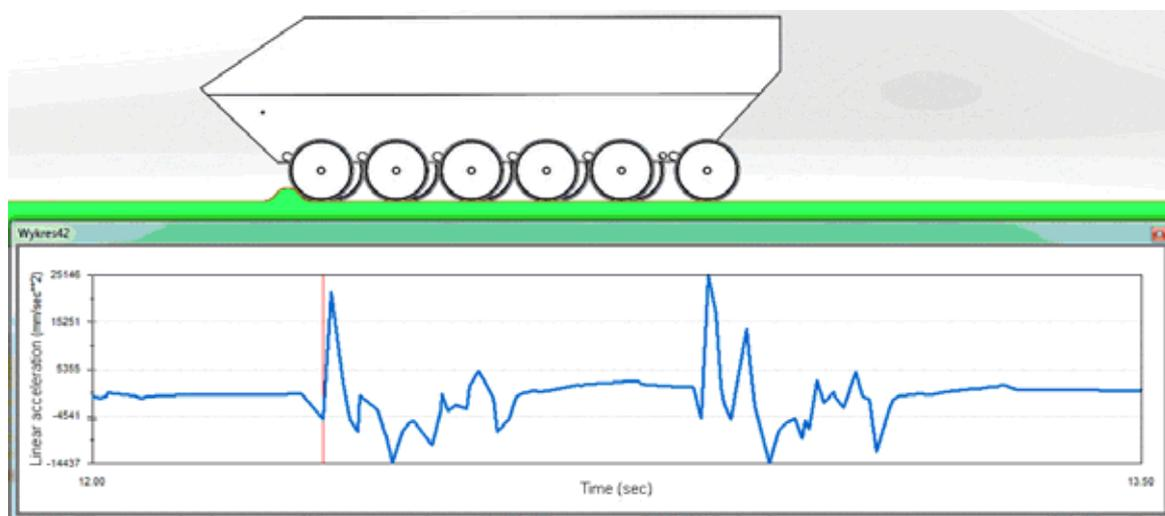
**Fig. 11. Graph of the acceleration of the front edge of the hull (vehicle shown just before reaching the obstacle, maximum acceleration  $25.146 \text{ m/s}^2$ )**
