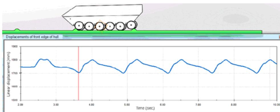
**Fig. 17. Graph of the displacement of the front edge of the hull (vehicle shown just before reaching the 2nd bump)**
