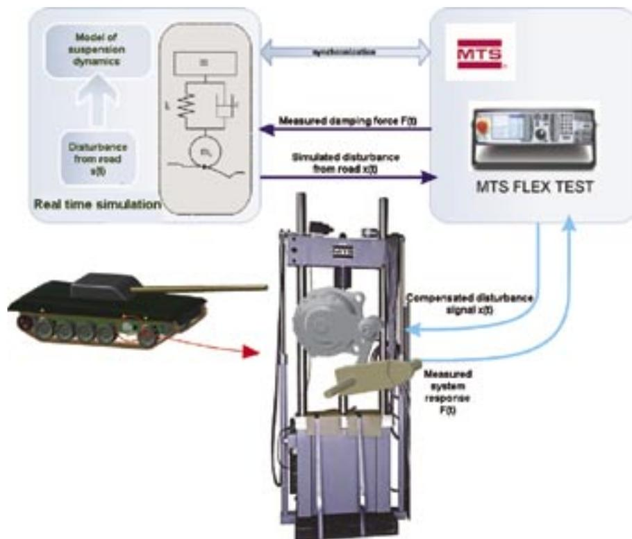
**Fig. 5. Example of a flowchart of a hardware in the loop simulation [3]**
