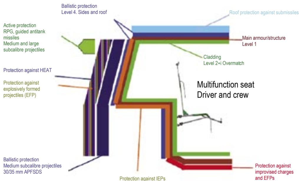
**Fig. 8. Cross-section of the hull of a special vehicle equipped with a complex system of additional armour shields**
