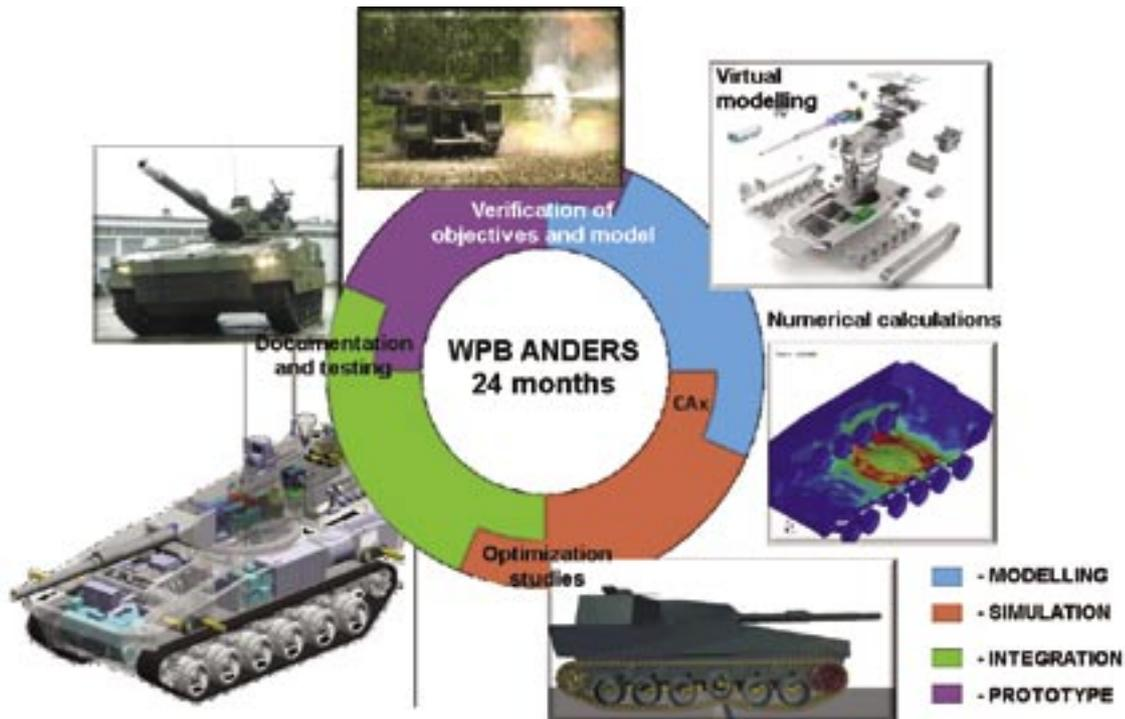
**Fig. 1. Advanced methods of design and modelling applied in the ANDERS project**
