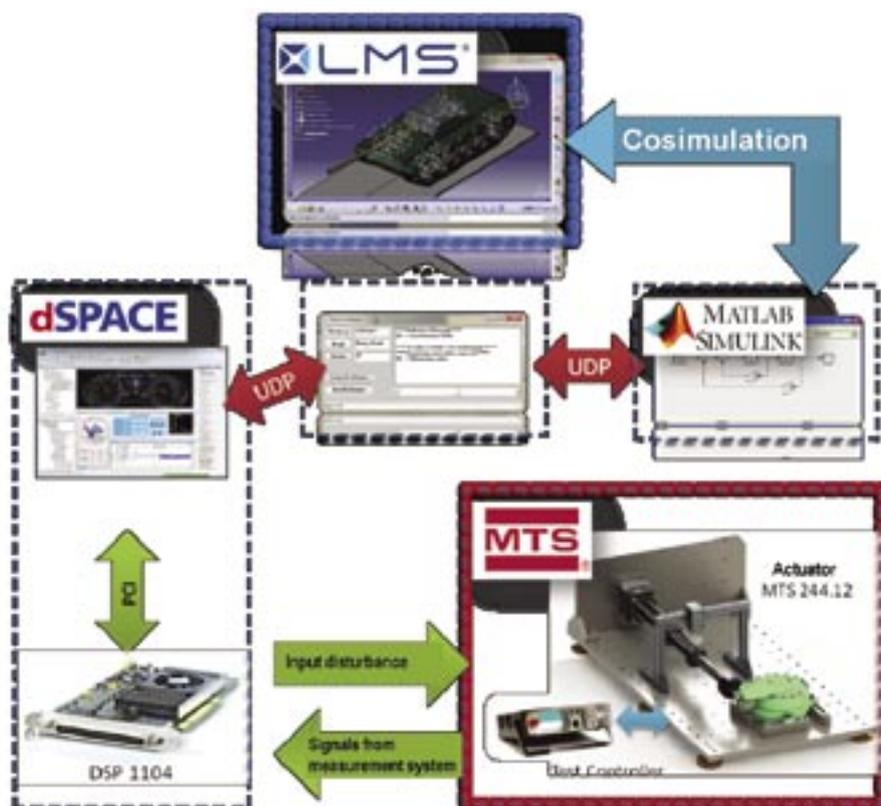
**Fig. 6. Hardware in the loop simulation using a dSpace Real Time board [3]**
