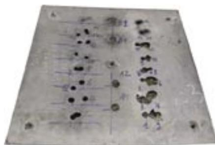
**Fig. 12. Testing of steel armour resistance to multiple hits: left – nanostructured steel, right – RHA armour steel**
