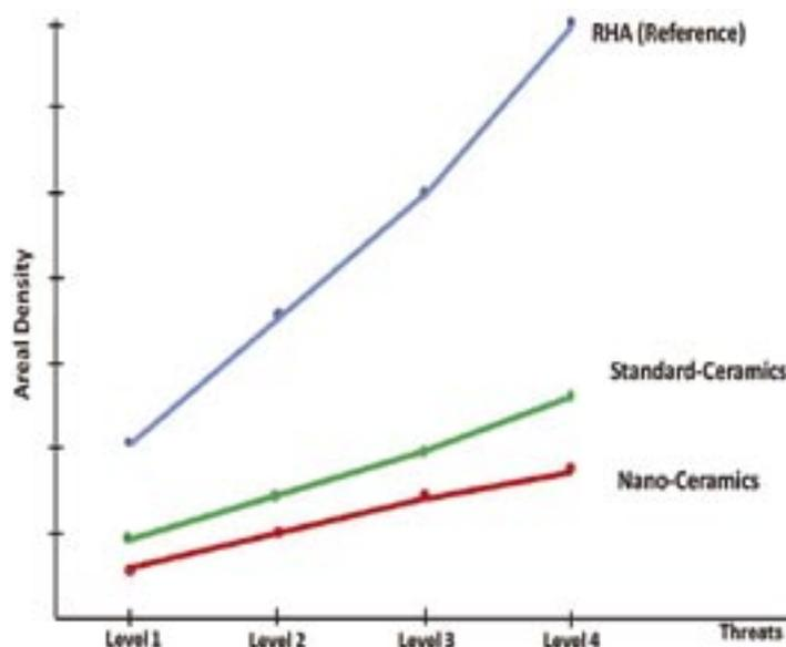
**Fig. 11. Comparison of the unit weight of armour made of RHA steel, ceramic armour and nanostructured ceramic armour in relation to the level of ballistic protection (STANAG 4569)**
