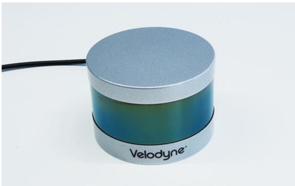
**Fig. 3. 3D LiDAR from Velodyne (photo by OBRUM sp. z o.o.)**
