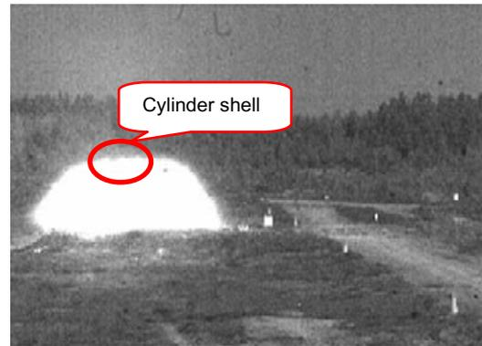
**Fig. 5d - 0.2695 s after decompression - flying cylinder fragment spotted**
