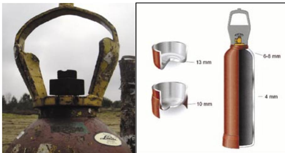
**Fig. 2. Acetylene cylinder used in the tests**
