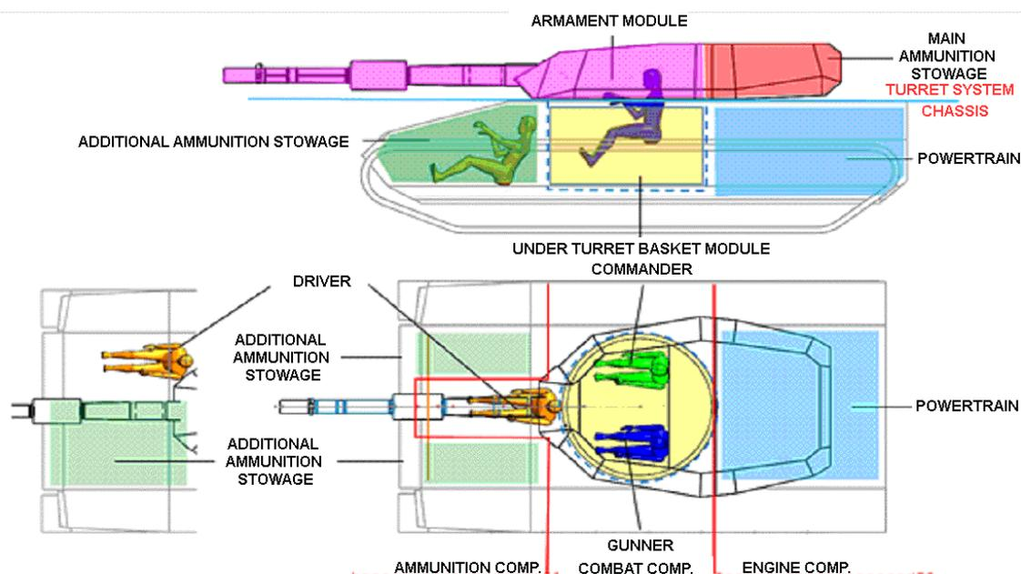
**Fig. 3. General structure of a tracked combat vehicle with the engine compartment at the rear**
