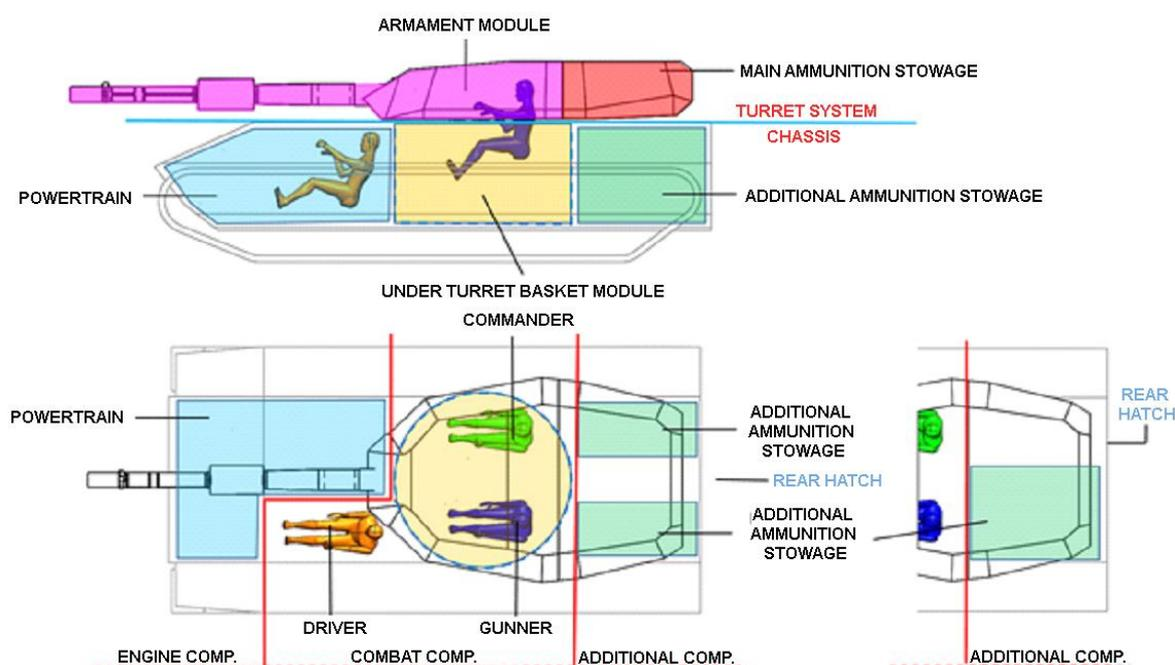
**Fig. 1. General structure of a tracked combat vehicle with the engine compartment in the front**
