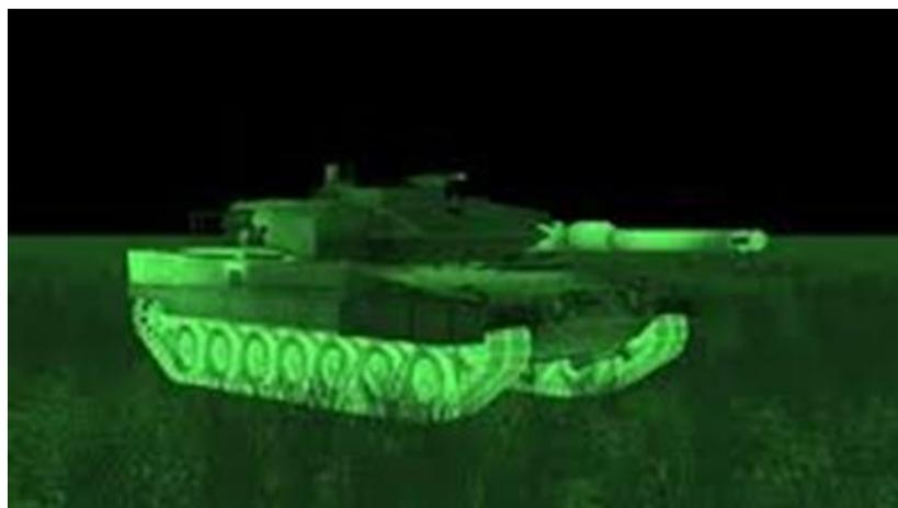
**Fig. 4. Thermovision camera image of a combat vehicle with the powertrain at the rear**
