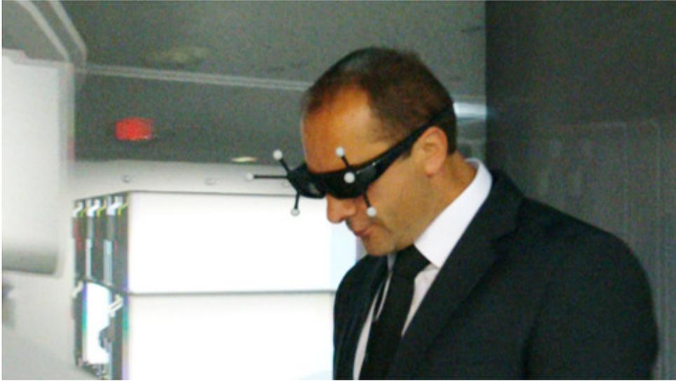
**Fig. 5. Headset with passive markers (photo by OBRUM)**
