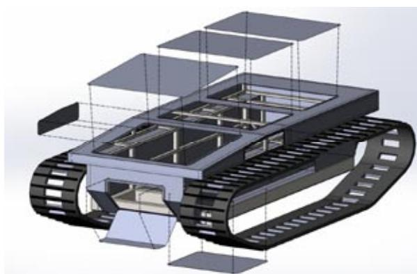
**Fig. 7. Chassis body – inspection doors and covers**
