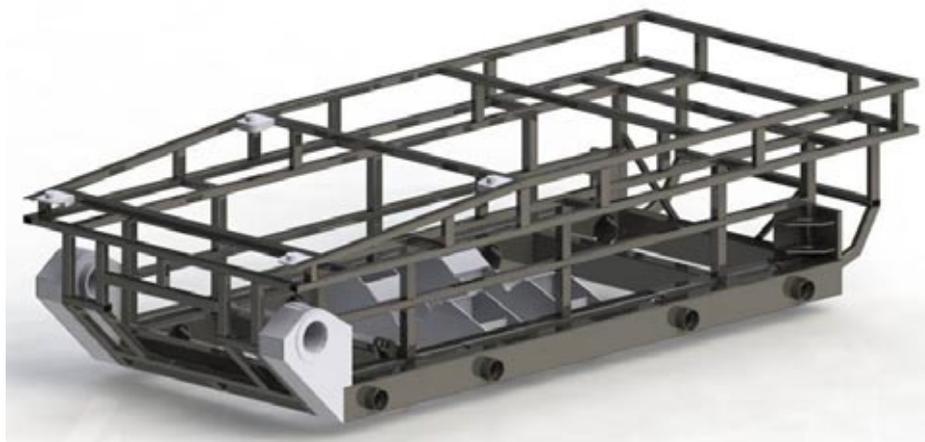
**Fig. 8. Chassis body – framework**
