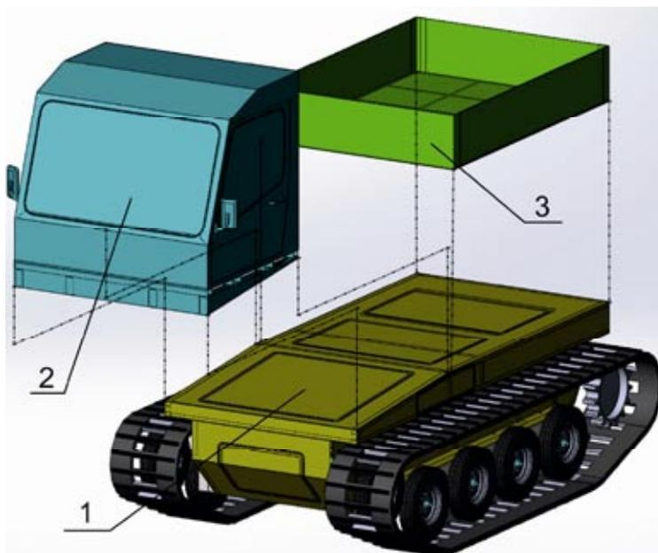
**Fig. 6. General structure of the WIPH vehicle**
