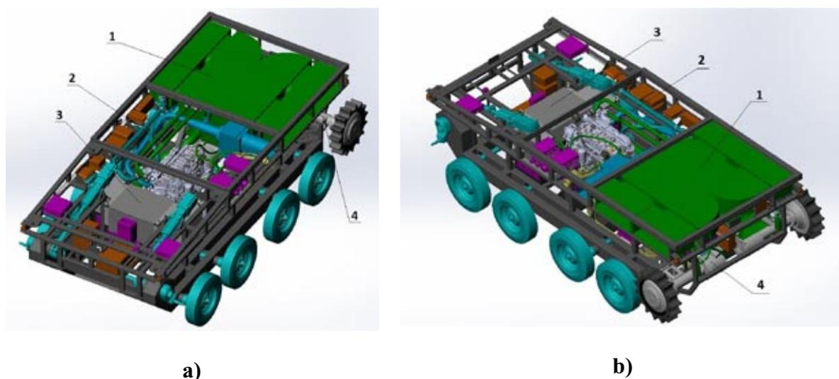
**Fig. 9. Arrangement of the main drive components inside the chassis**
