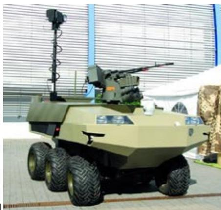
**Fig. 5. LEWIATAN ZS unmanned vehicle**
