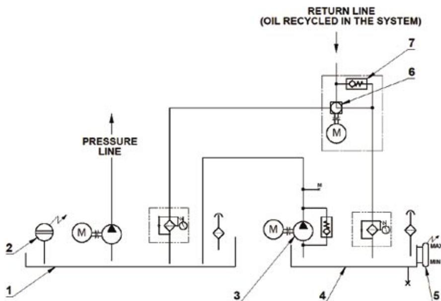
**Fig. 1. Block diagram of the compensation system**
