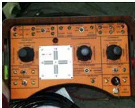
**Fig. 5. Control panel for radar station levelling system**
