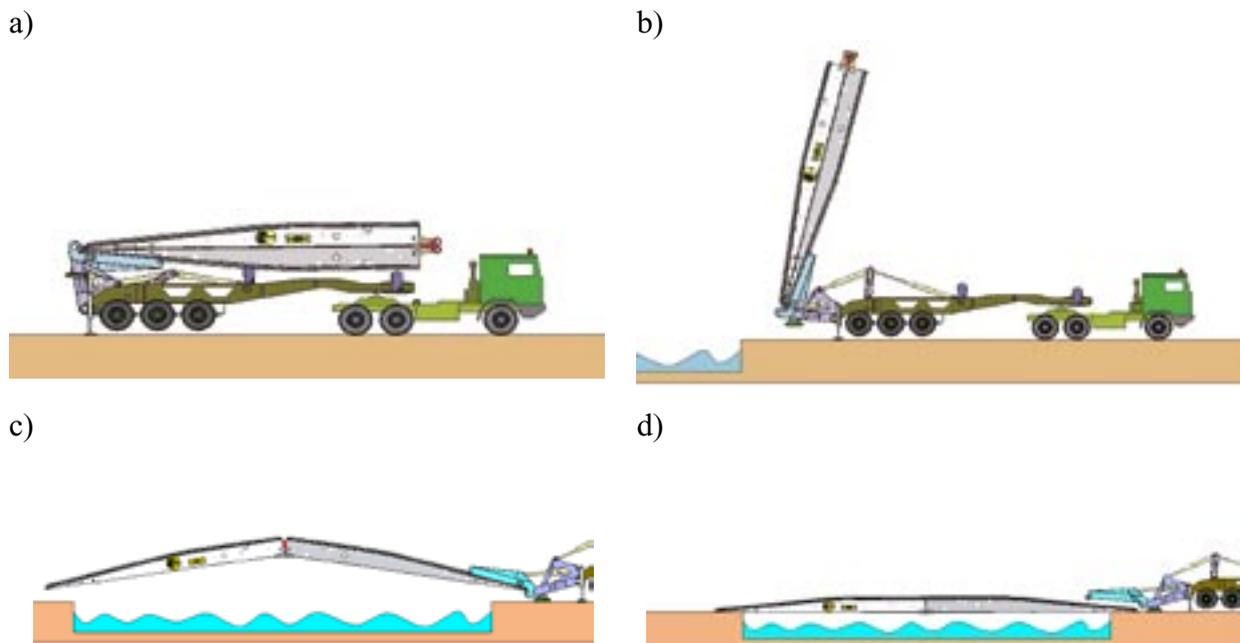
**Fig. 2. Phases of launching the MS-20 bridge**
