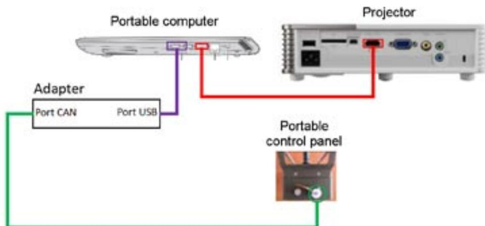
**Fig. 7. Interaction between the S-MS-20 simulator and the portable control panel**
