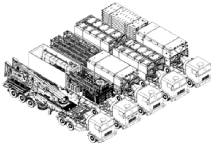
**Fig. 4. MS-40 support bridge on wheeled chassis**
