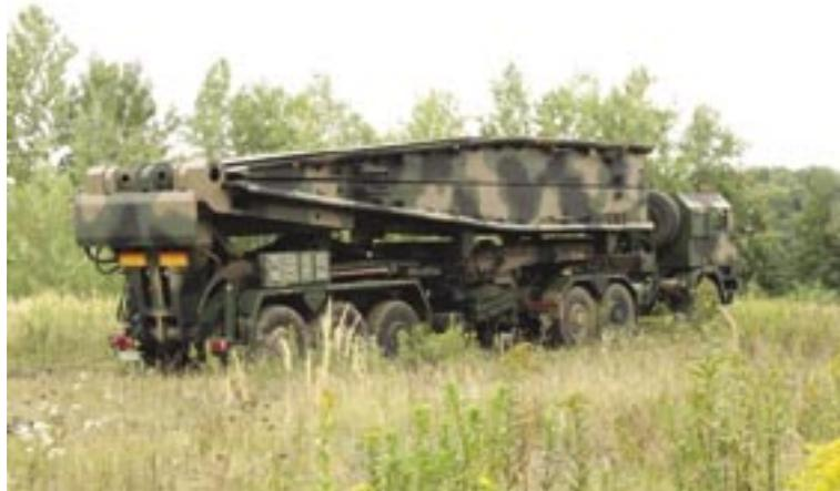
**Fig. 1. MS-20 support bridge on wheeled chassis**
