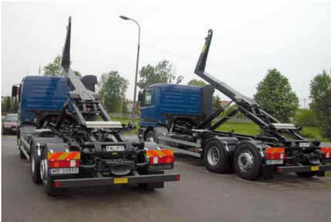
Fig. 9. Palfinger Power system installed on a wheeled chassis
