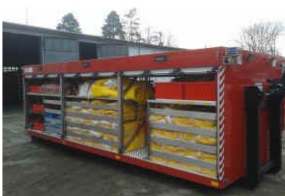
Fig. 4. Container with barriers
