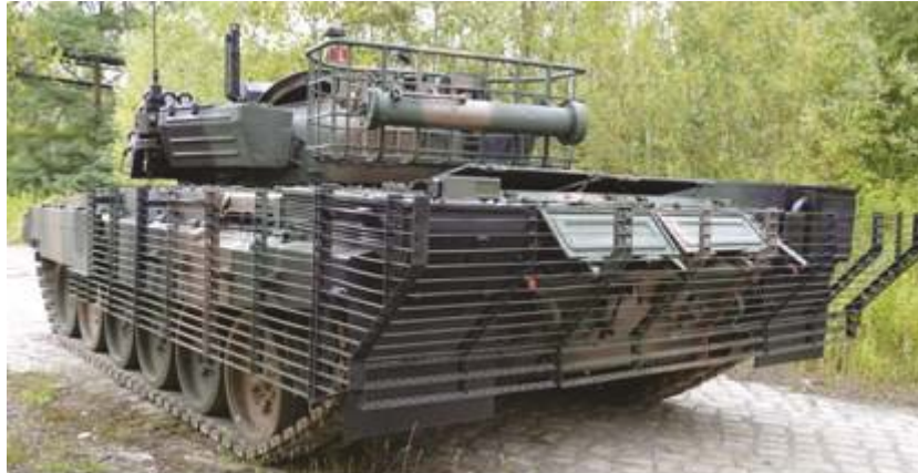
Fig. 4. Bar armour installed on the PT-91M2 tank
