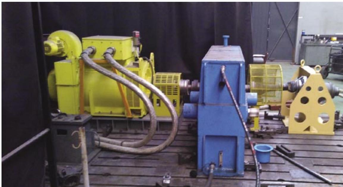
**Fig. 1. Final drive test stand with no working load**
