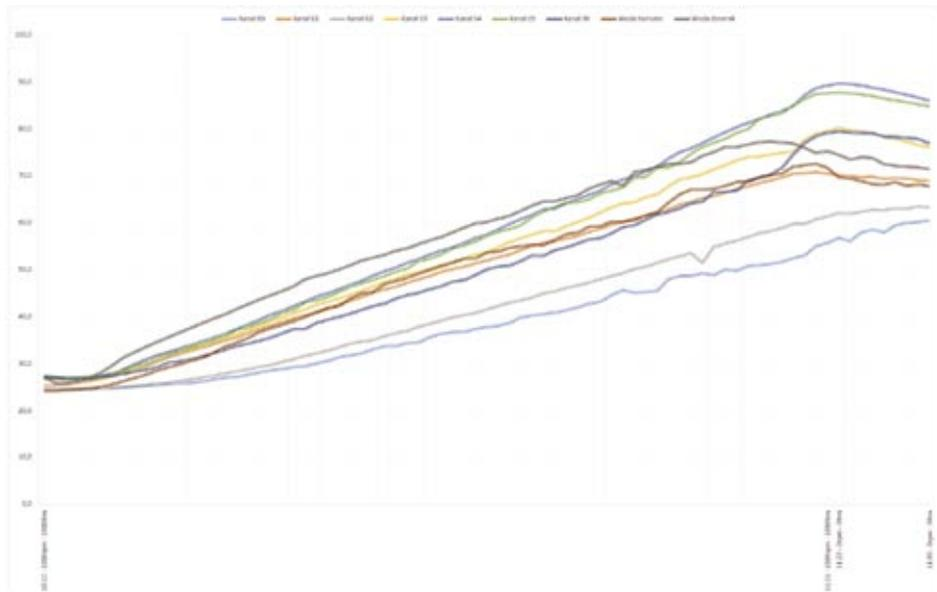
**Fig. 8. Temperature changes recorded in the modified right-hand final drive**
