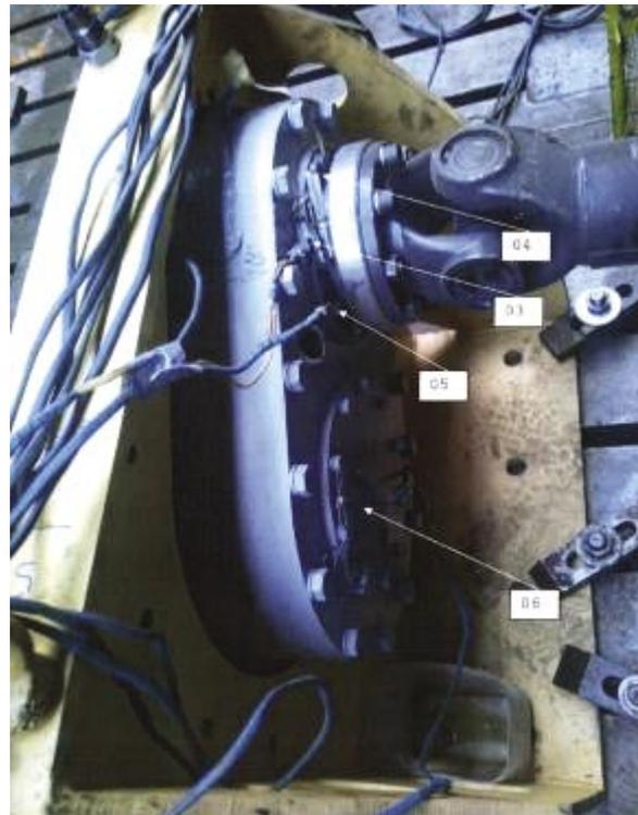
**Fig. 3. Arrangement of temperature measurement points**
