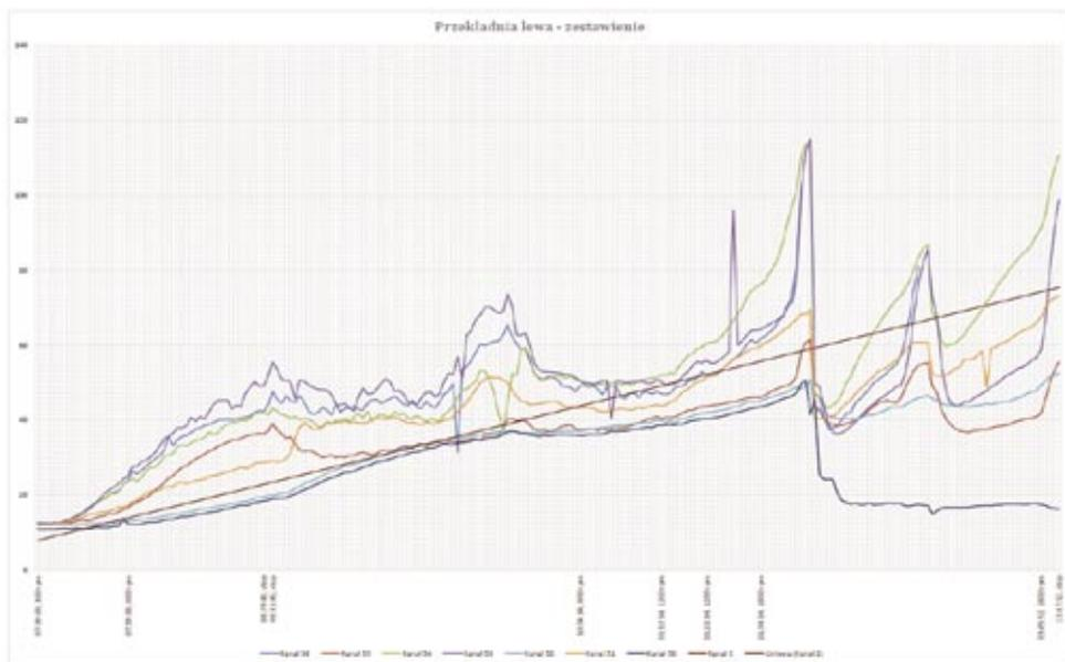
**Fig. 6. Temperatures recorded at measurement points of the right-hand final drive tested under no load**
