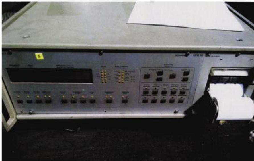
**Fig. 4. UPM60 temperature recorder**
