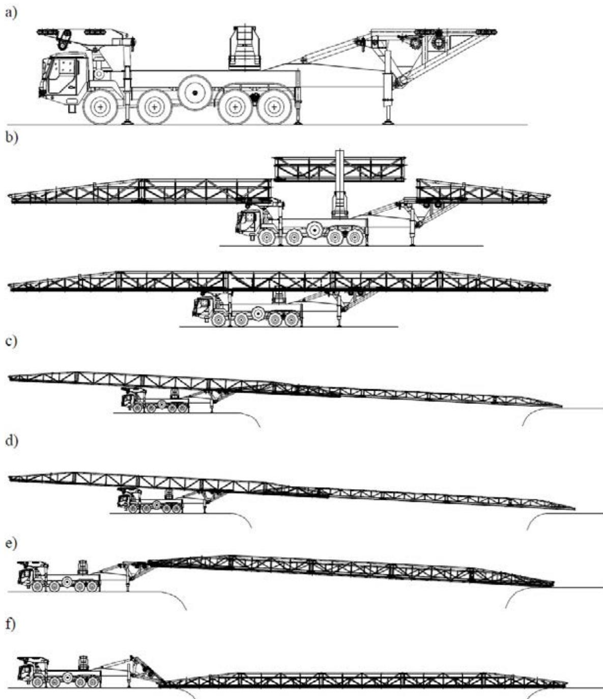
**Fig. 5. Subsequent stages of the launching of an HZQL51m bridge (in accordance with [4] and [5]):**
