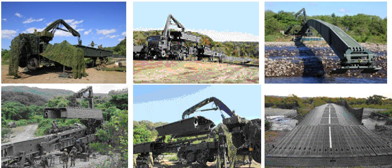
**Fig. 10. Main operations in the Type 07 bridge launching procedure [11, 12]**
