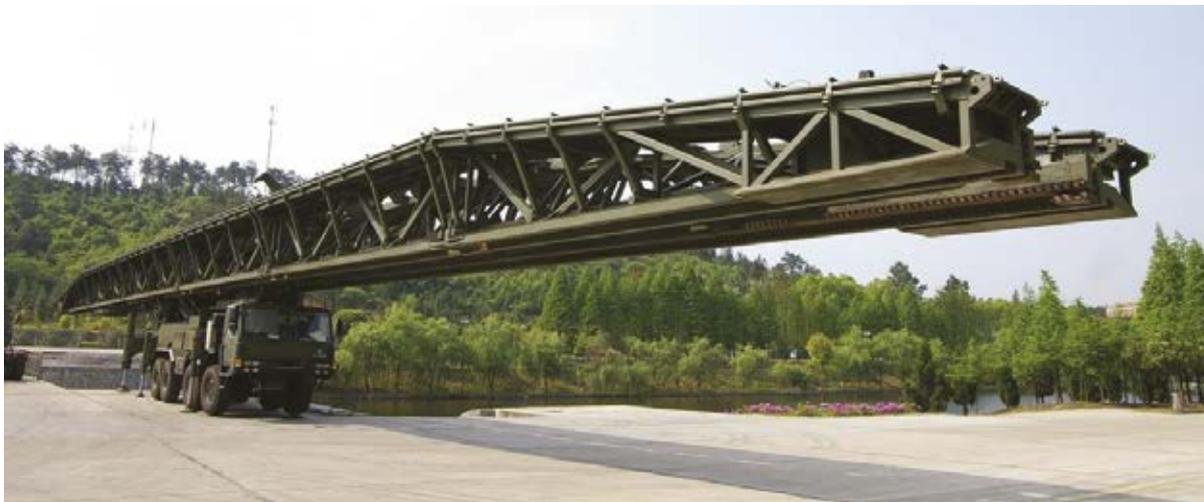
**Fig. 2. View of HZQL51 bridge span being deployed [4]**
