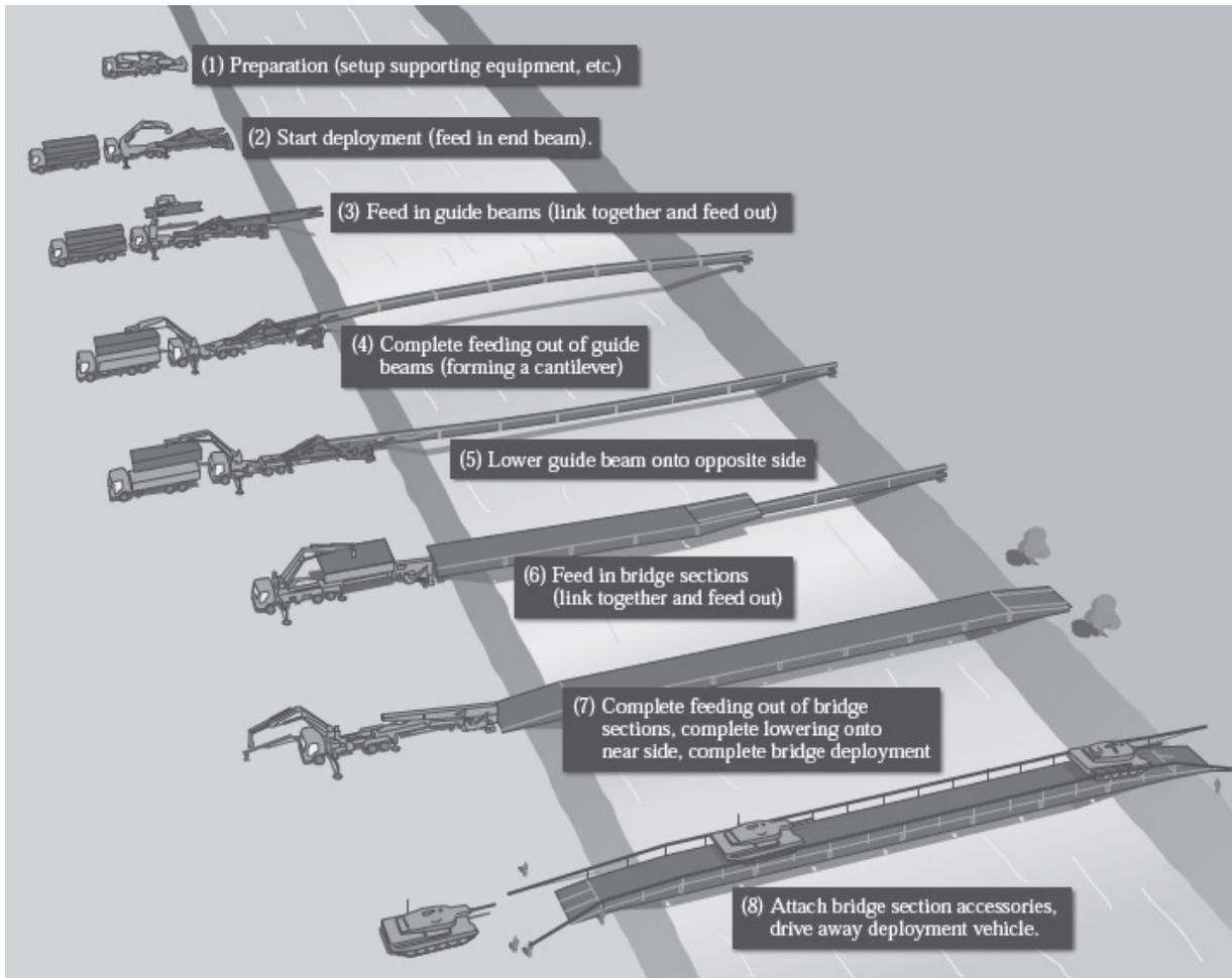
**Fig. 9. Launching of the Type 07 bridge over an obstacle [7]**
