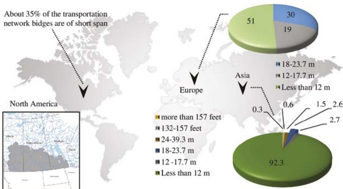
**Fig. 1. Terrain obstacle gap widths and their distribution in various regions of the world [2]**
