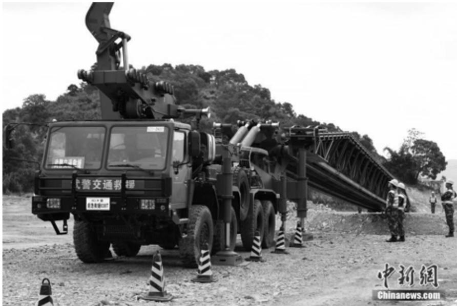
**Fig. 6. Launching operation, setting the HZQL51 m span over an obstacle [6]**
