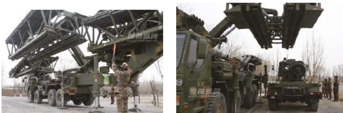
**Fig. 4. Launching operation, arranging the middle section of the span on the layer vehicle [6]**
