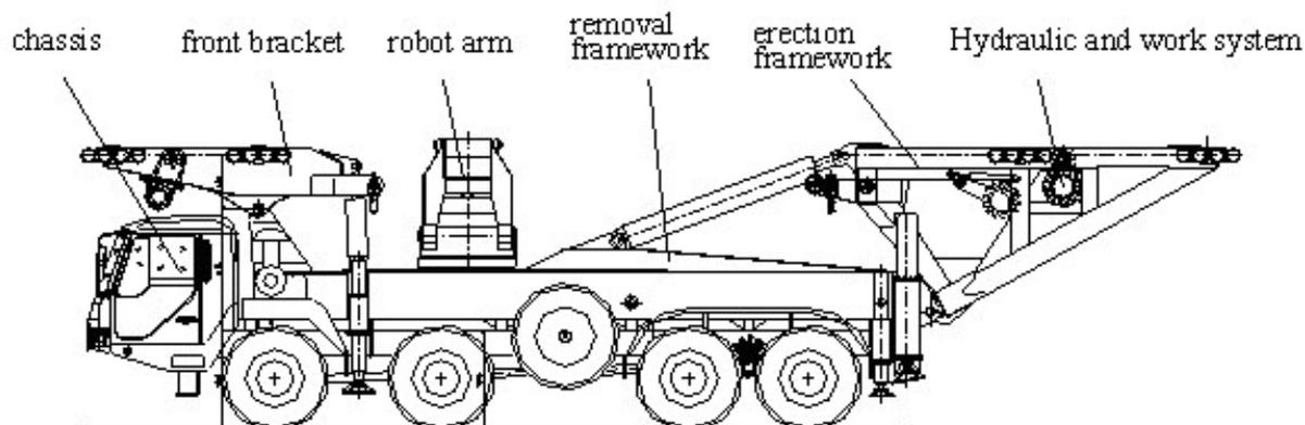
**Fig. 3. Schematic of the launching vehicle [5]**
