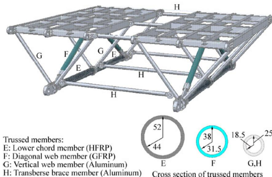
**Fig. 13. Hybrid truss made of aluminium and composites [18]**
