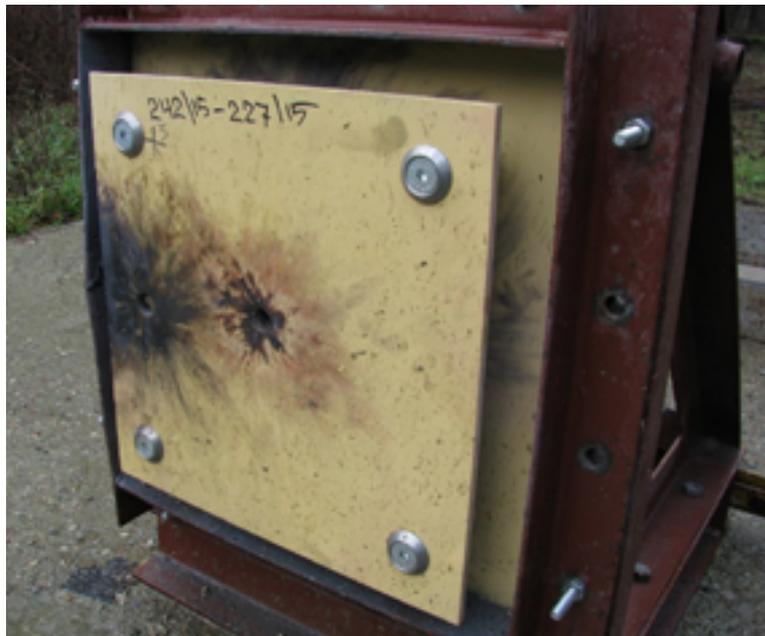
**Fig. 1. Sample piece of armour installed on the test stand**
