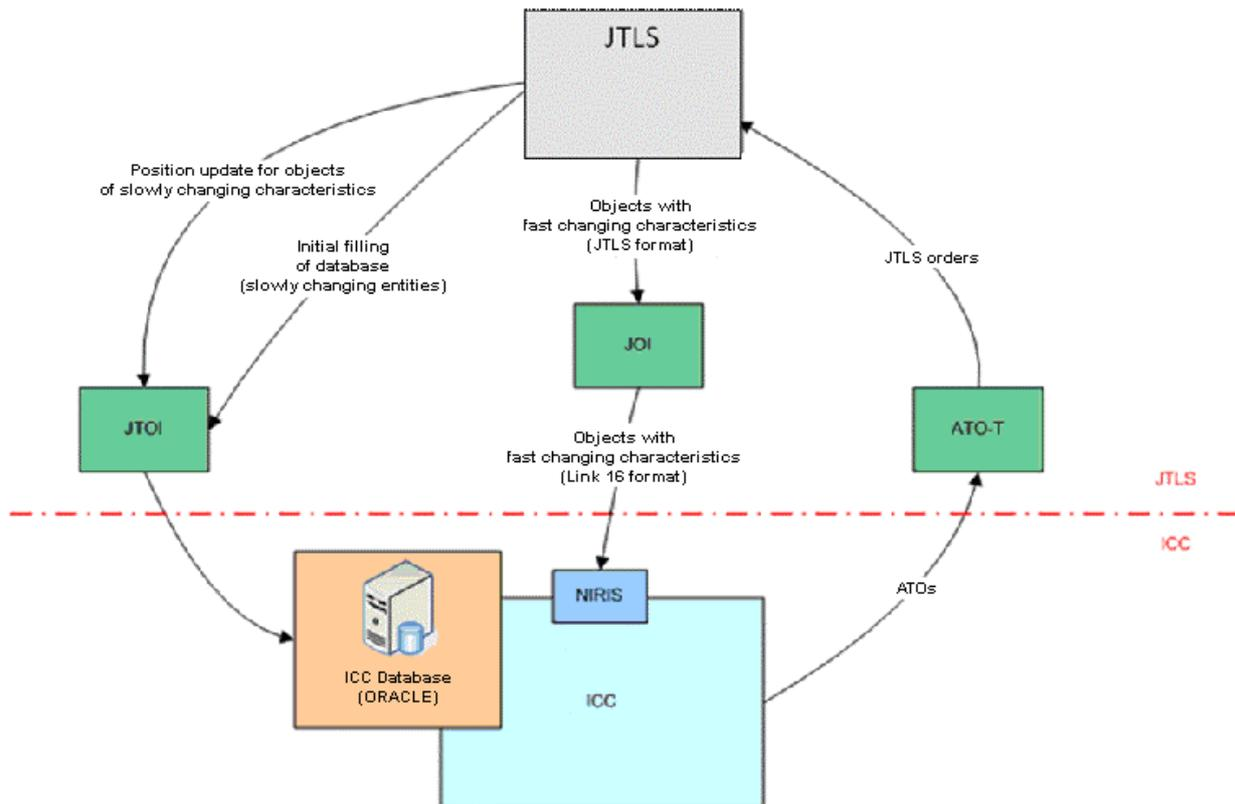
**Fig. 4. JTLS and ICC interactions during CAX**
