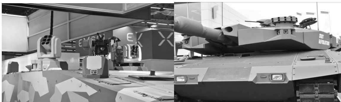
Rys 4. ASOP LEADS-150 na transporterze opancerzonym i system ROSY na Leopard MBT Revolution
