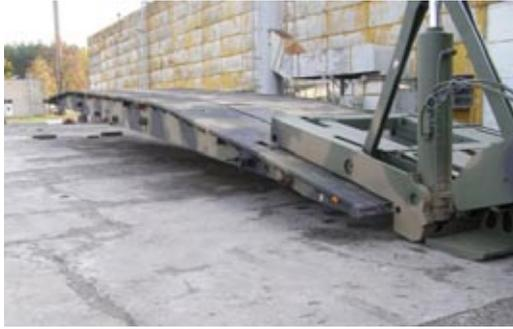
**Fig. 7. Moment corresponding to emergency stopping of the span 1 m above the ground**
