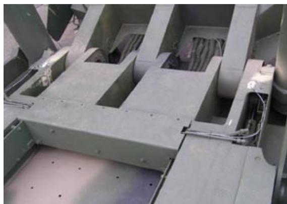
**Fig. 6. View of strain gauges arrangement on the bridge layer**
