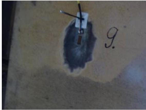
Gauge t9 – lower left chord of the middle segment of the main span
