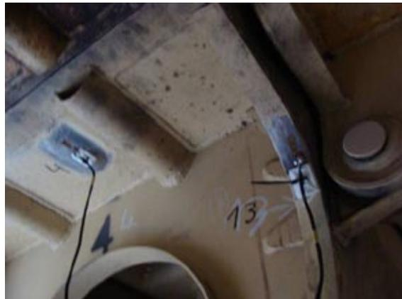
Gauges t4 and t13 – deck underside and vertical wall of the middle segment of the main span
