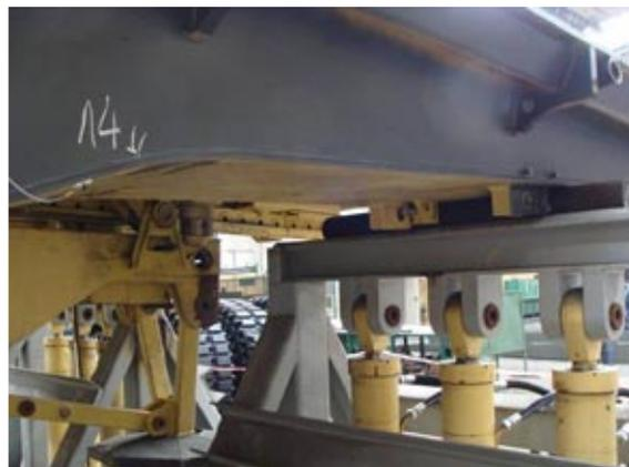
Gauge t14 – lower right chord of the approach segment of the main span
