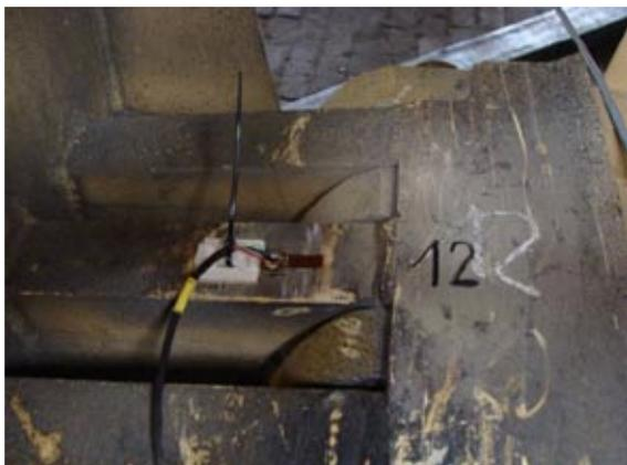
Gauge t12 – lug beside the bolt of main span
