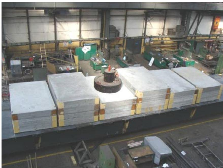
**Fig. 11. Span loaded with weights during the "U" test - wheeled vehicle load**
