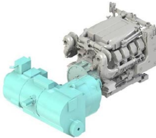
Fig. 1. Conventional drive system of the ANDERS Fire Support Vehicle [17,18]
