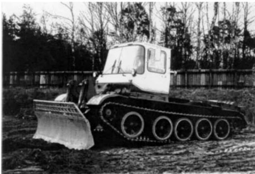
**Fig. 4. ATS tractor based on T-55 tank chassis**
