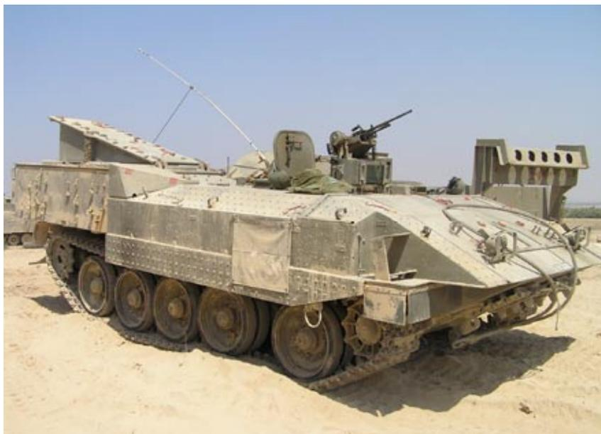
**Fig. 2. ACHZARIT APC based on T-55 chassis**
