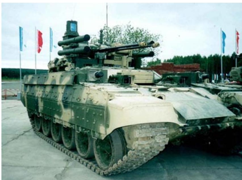
**Fig. 3. BMPT – Russian heavy fighting support vehicle based on T-72 MBT chassis**
