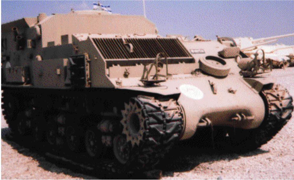
**Fig. 1. M4A1-based medical evacuation vehicle**
