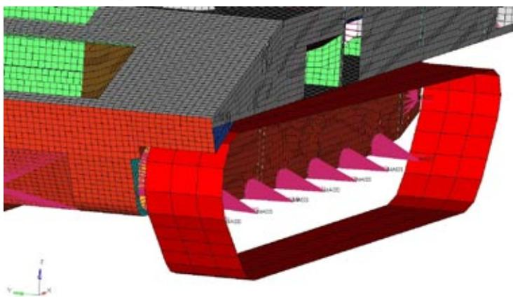
**Fig. 10. Connection between suspension and body effected by means of interpolation constraints**
