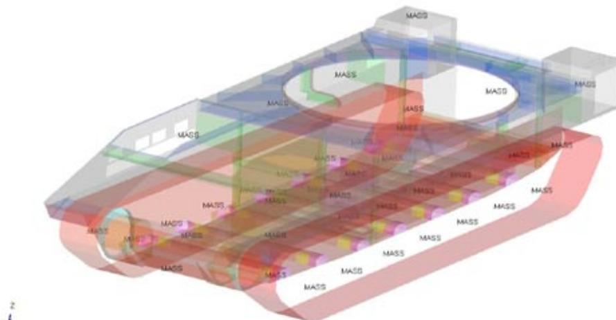
**Fig. 9. Arrangement of concentrated masses in the numerical model**
