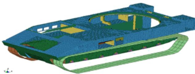
**Fig. 2. Numerical model of the KRAB vehicle – general view**
