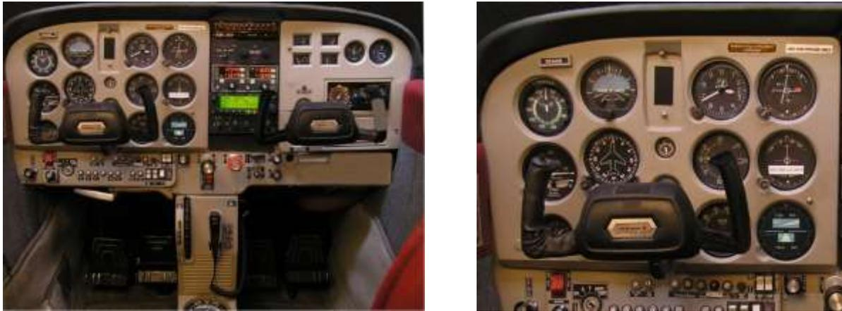
**Fig. 3. CDI indicators installed in flight simulator**
