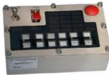
**Fig. 10. View of the system control panel (PCS) of HITFIST 30P turret in AMV Rosomak**
