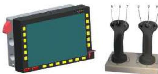
Fig. 8. View of the display and the control console of HITFIST 30P turret in AMV Rosomak
