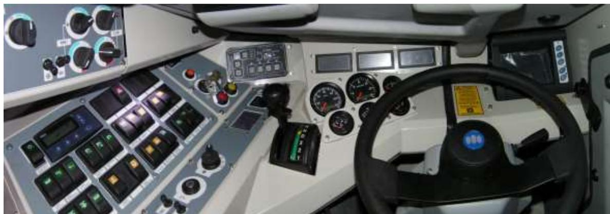
**Fig. 1. Interior of AMV Rosomak – driver's compartment**
