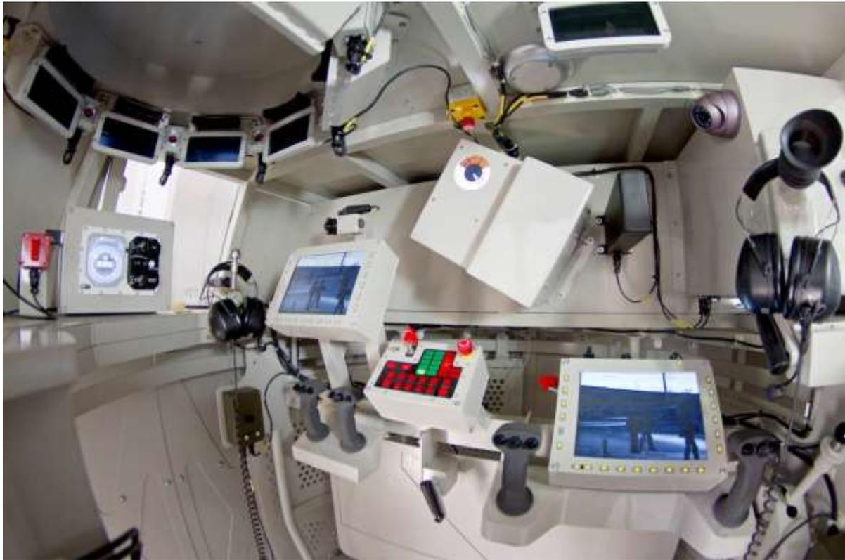
**Fig. 4. Interior of SKMB module, gunner's and commander's stand**
