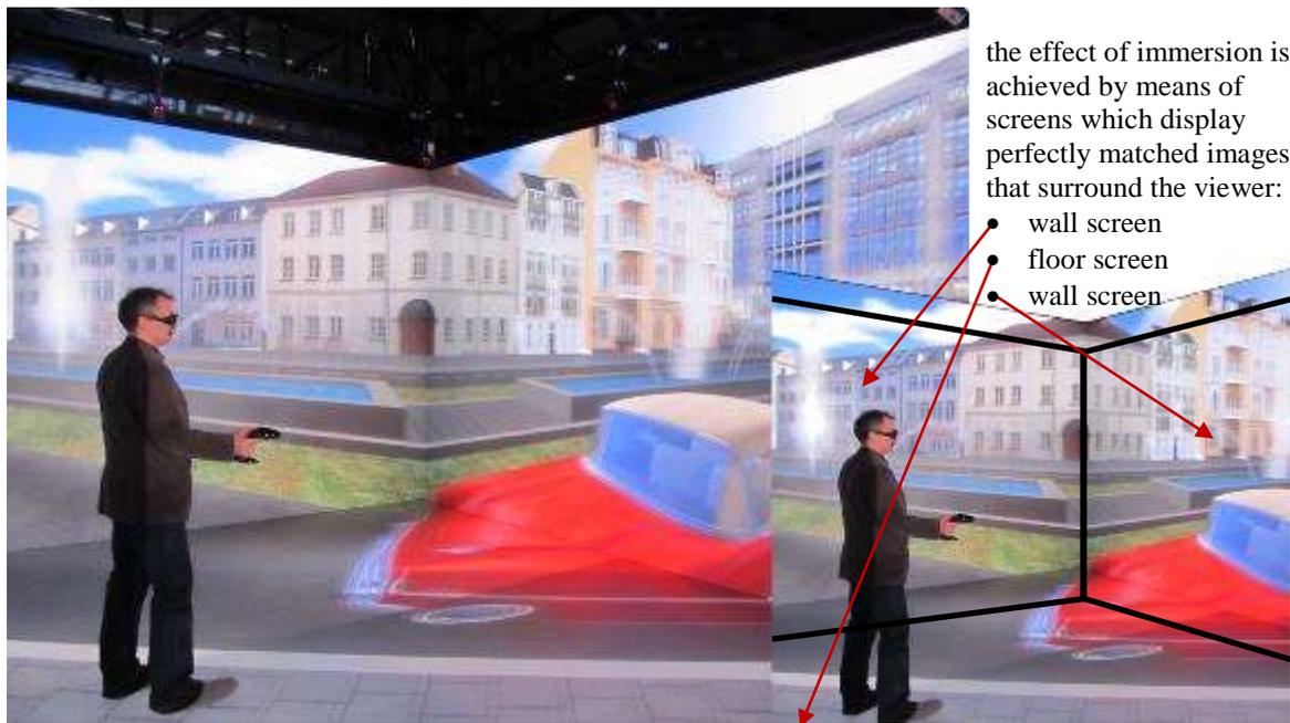
**Fig. 2. An example of a virtual cave [10] and its operating principle** (photo by A. Mazikowski)
