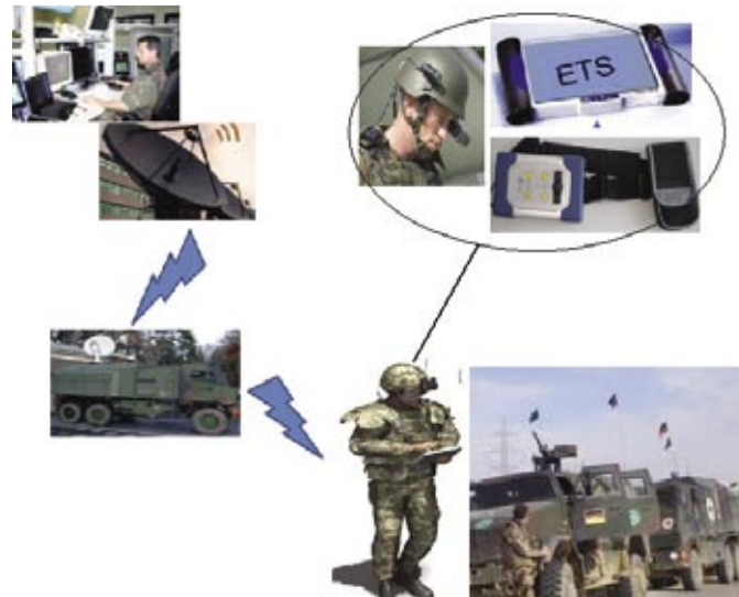
Fig. 2. The concept of telemaintenance system in German Land Forces to support expedient repairs during combat operations [11]
