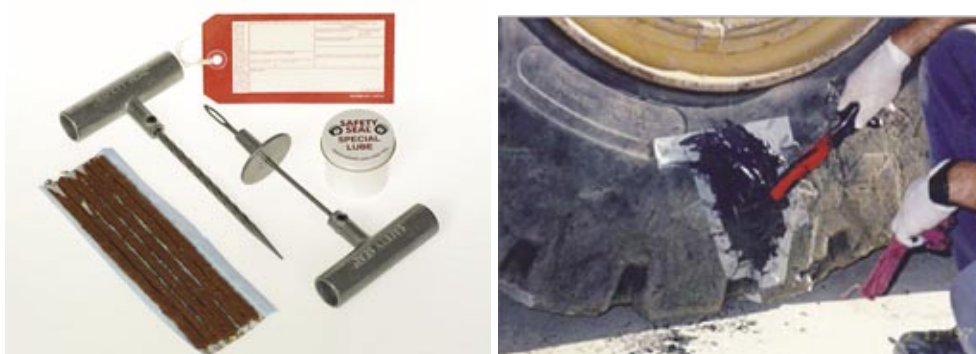
Fig. 8. Methods of tire repairs with the use of the special kit (left) and adhesive composites (right)
