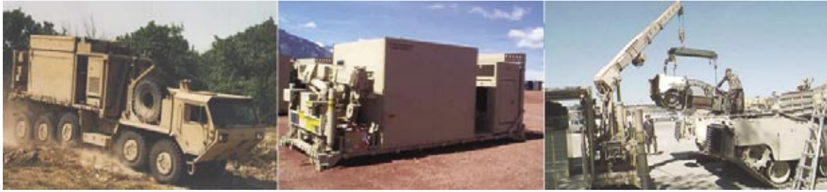
Fig. 2. FRS on a HEMTT-type vehicle during transportation (left), working post after removing from the transporting vehicle (middle) and during repair works (right) [5]
