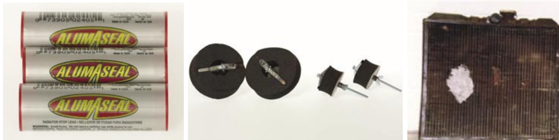
Fig. 9. Methods of small holes repair with a sealant (left) and large holes repair with plugs (middle) and adhesive composite (right)
