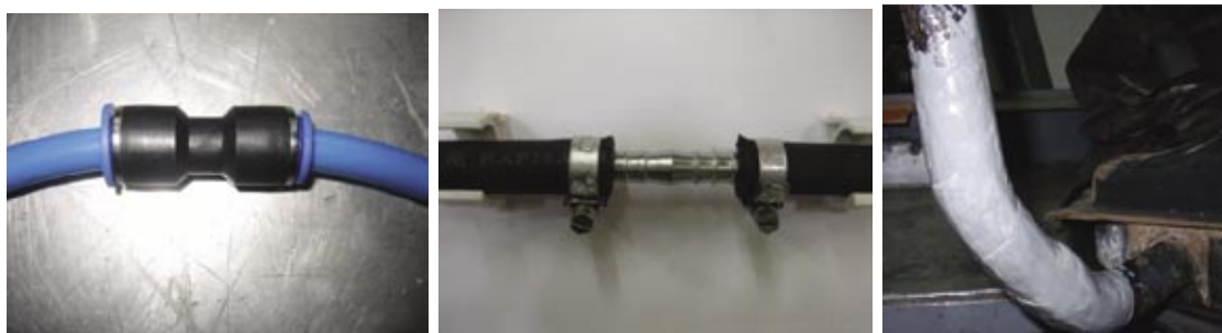
Fig. 6. Sample methods of repairing lines by fast-joints (left), clamps (middle) and adhesive composites (right)
