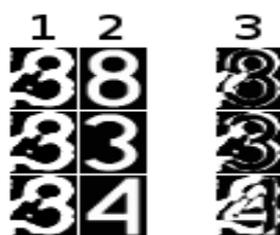
**Fig. 17. Illustrative visualisation of the principle of the template comparison method (average grey channel width for the digit 8 is lowest in this case)**
