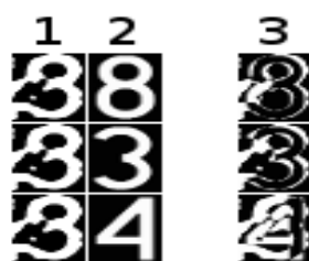
Fig. 17. Illustrative visualisation of the principle of the template comparison method (average grey channel width for the digit 8 is lowest in this case)
