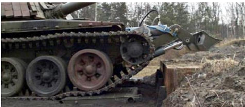
**Fig. 5. Bank support of the PMC - LEGUAN bridge during preliminary testing**
