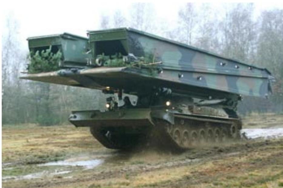
**Fig. 2. KMW LEGUAN bridge (LEOPARD 1 chassis with seven pairs of road wheels)**
