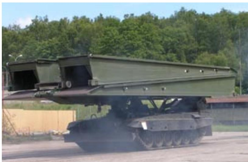
**Fig. 10. PMC – LEGUAN assault bridge (PT-91M chassis with six pairs of road wheels)**
