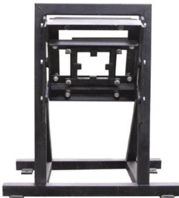
Fig. 4. Stand for testing samples of add-on armour
