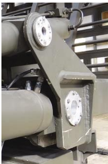
Fig. 1. Fragment of supporting framework of JBR-15 radar station
