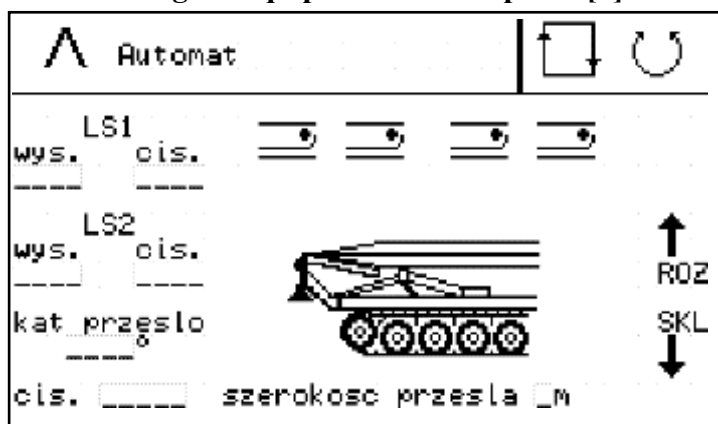
9.1. Bridge span in transport position – sequences 1-2
