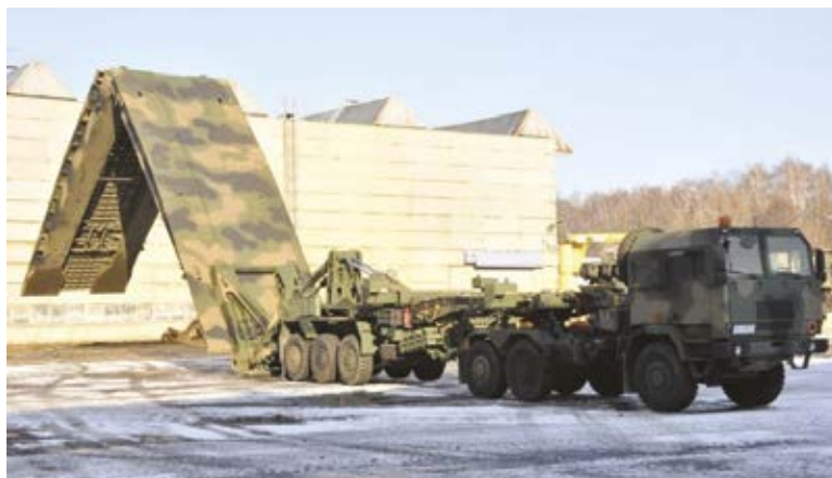
Fig. 1. Launching the MS-20 bridge span in open terrain [14]
