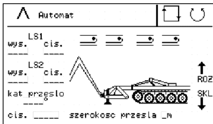
9.3. Span unfolding – sequences 4-6
