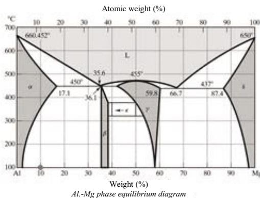
Fig. 1. Al-Mg phase diagram [4]
