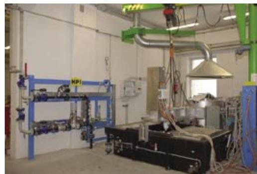
**Fig. 3. Line for semi-continuous casting magnesium alloy billets**
