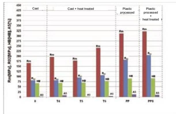
Fig. 2. Graphic representation of mechanical properties of AZ91 alloy depending on the type of processing [6]
