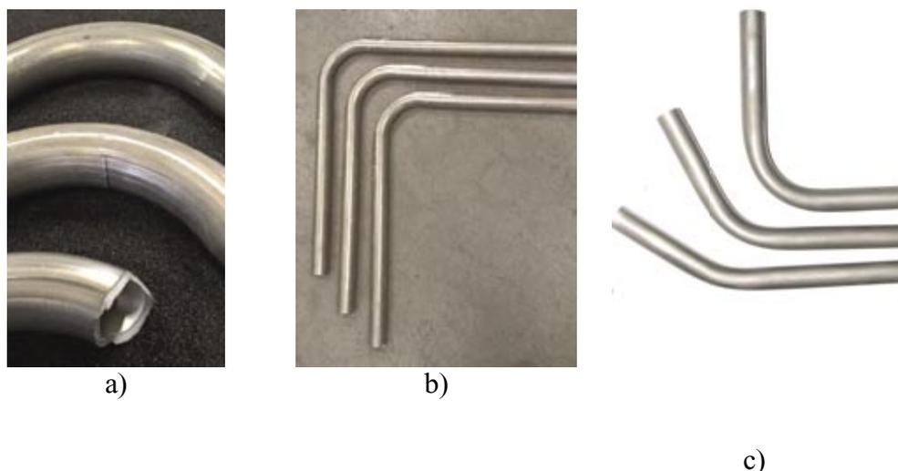
**Fig. 9. Tube bending tests**
