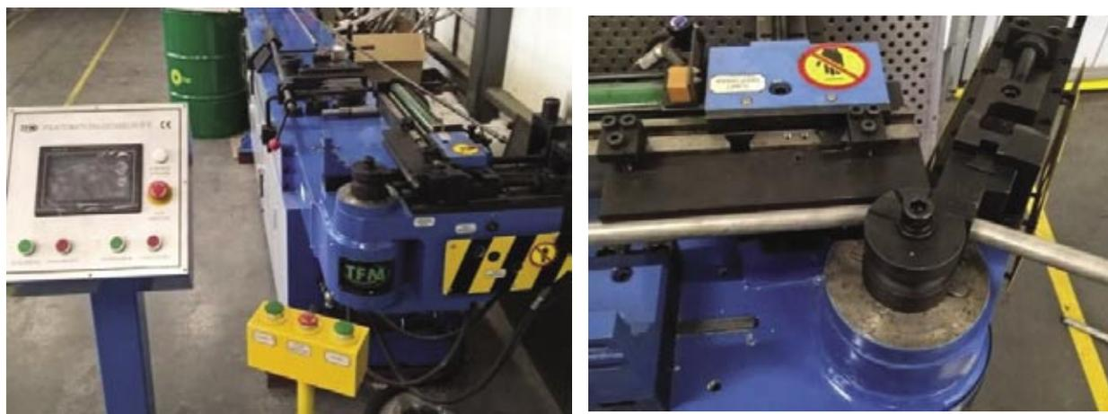
Fig. 5. A GM-38NCB bending machine with tooling for bending magnesium alloy tubes
