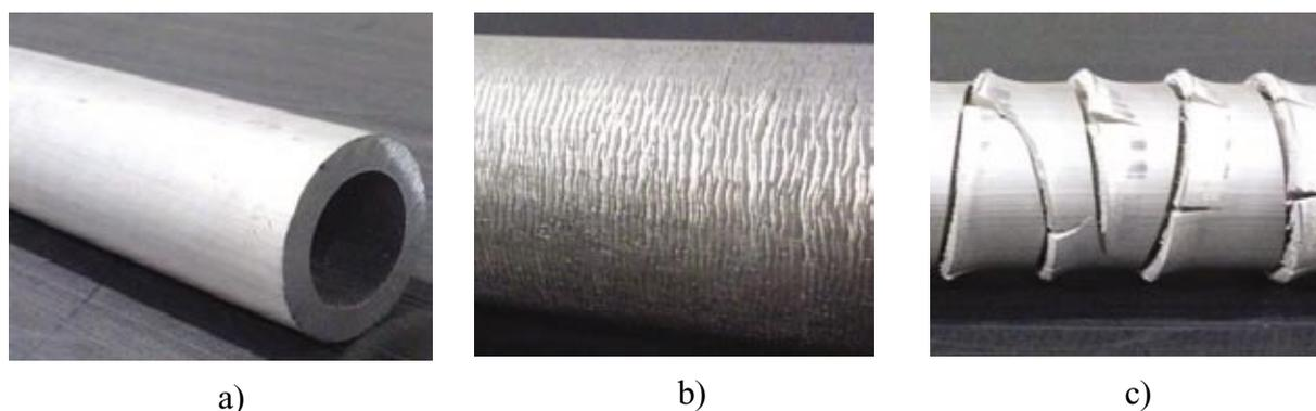
**Fig. 7. Examples of surface types of extruded products**
