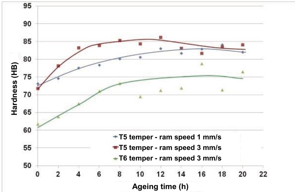
**Fig. 8.** Curves of natural and artificial ageing of the AZ80A magnesium alloy at 175°C
