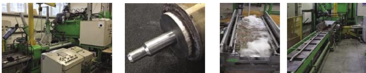
**Fig. 4. A 5 MN direct/indirect extrusion press with a piercer, "water wave" and run-out table**
