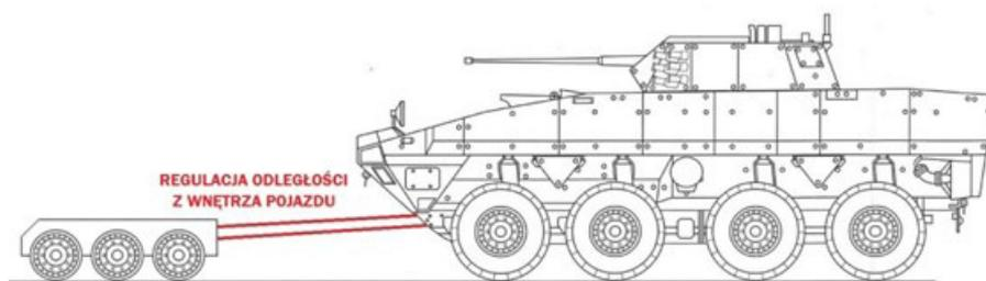
**Fig. 3. A proposed solution for the protection of crew against the method of fuse shifting**
