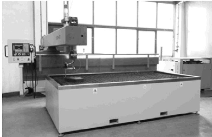
**Fig 5. View of the water jet cutter**
