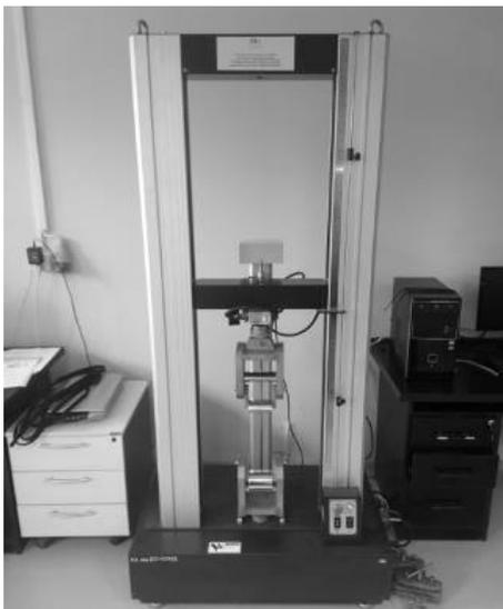
**Fig. 6. View of the QC-505A2 testing machine**
