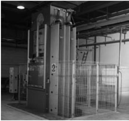
**Fig. 4. View of the PHM-2000E hydraulic press**
