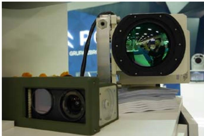
**Fig. 3. Optical upgrade kit for the LEOPARD 2A4/2A5 tank – rearview camera KDN-1T "Nyks" (left) and thermovision camera KLV-1 "Asteria" (right)**
