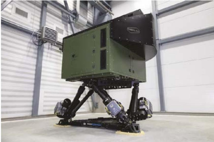
**Fig. 1. SJCL-6P simulator with a display system on a motion platform**
