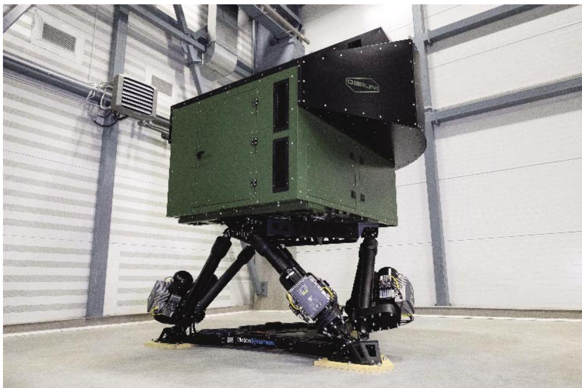
**Fig. 1. Leopard 2A4 tank driving simulator - SJCL
