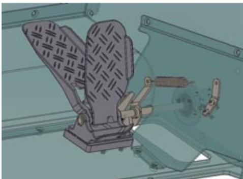
**Fig. 7. Accelerator pedal imitator**
