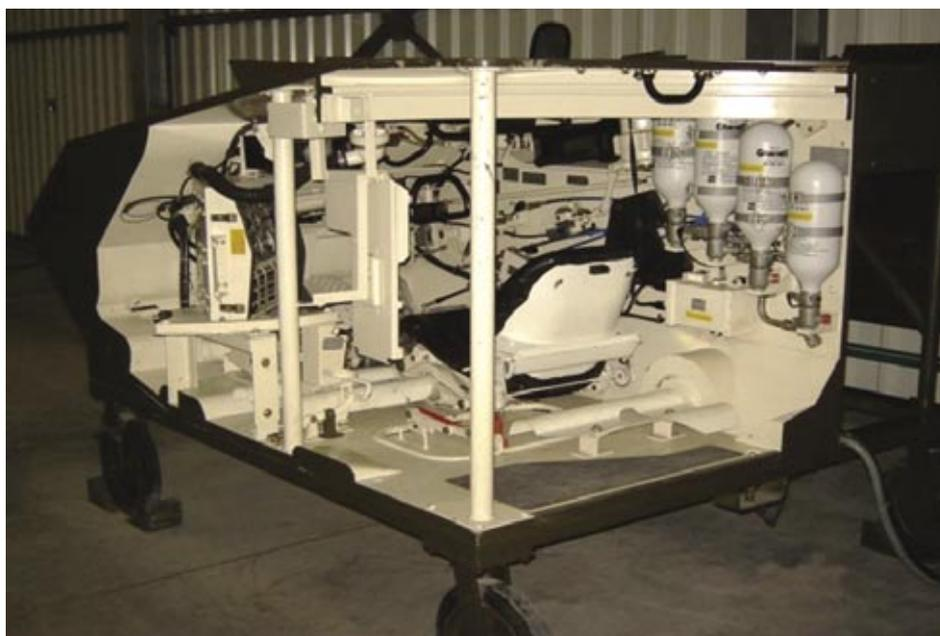
**Fig. 4. "CDT" type trainer device for drivers of the Leopard 2A4 tank [8]**
