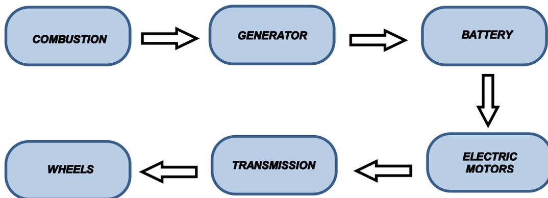
Fig. 1. Block diagram of a series hybrid drive
