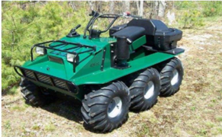
**Fig. 2. Hoot ATV 6x6 vehicle with 3 rigid axles**
