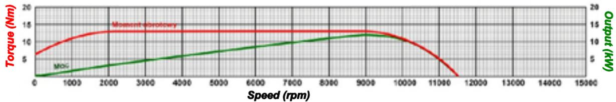
Fig. 3. Characteristics of the selected electric motor (supply voltage 72 V)
