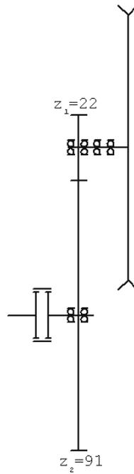
**Fig. 2. Kinematic diagram of final drive concept II**
