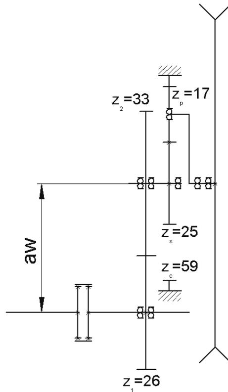
**Fig. 1. Kinematic diagram of final drive concept I**
