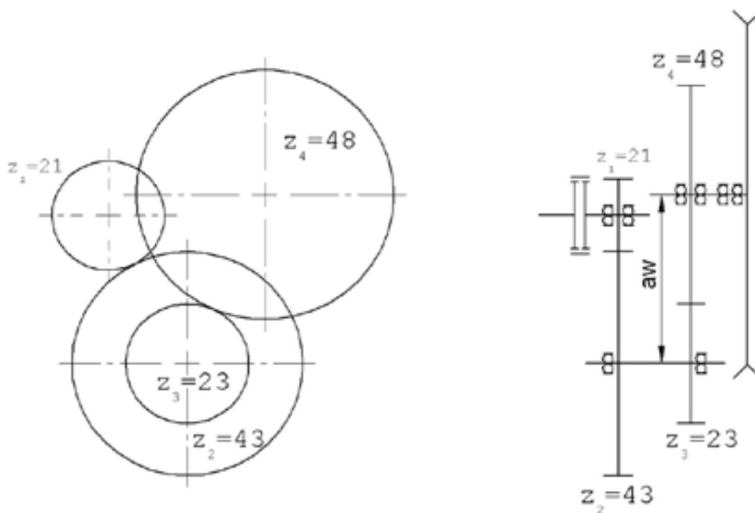
**Fig. 3. Kinematic diagram of final drive concept III**
