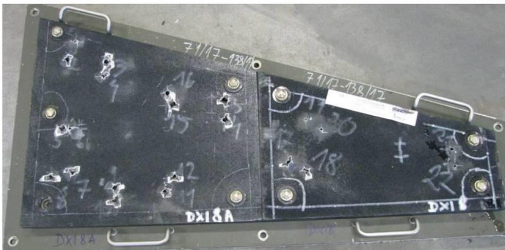
**Fig. 5. Armour demonstrator DXI8 (front)**
