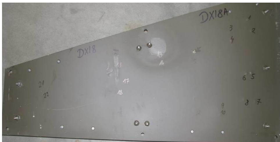
Rys. 6. Demonstrator opancerzenia DXI8 (tyl-blacha 8 mm)
