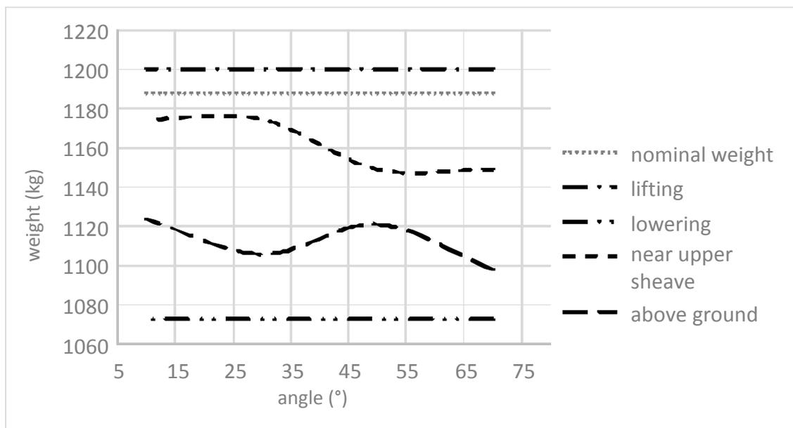
**Fig 5. Differences in indications for a 1,190 kg load**
