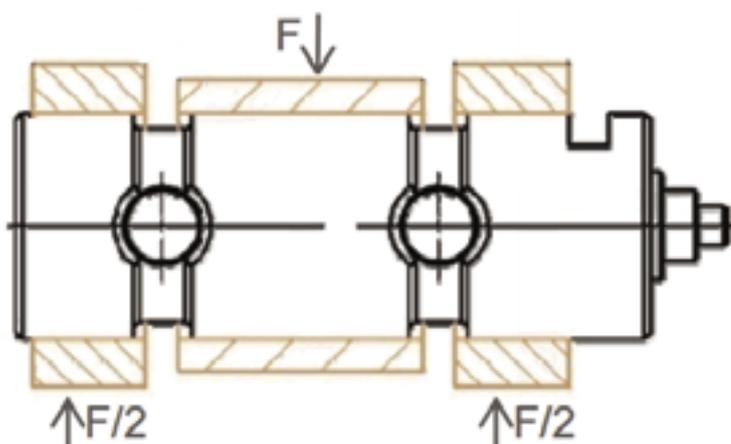
**Fig. 3. Operating principle of the BROSA 0201 force measuring pin [6]**
