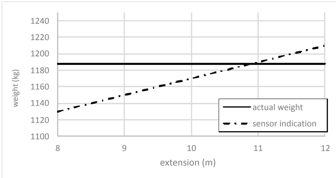
**Fig 6. Differences in indications for a 1,190 kg load at various degrees of telescopic boom extension**
