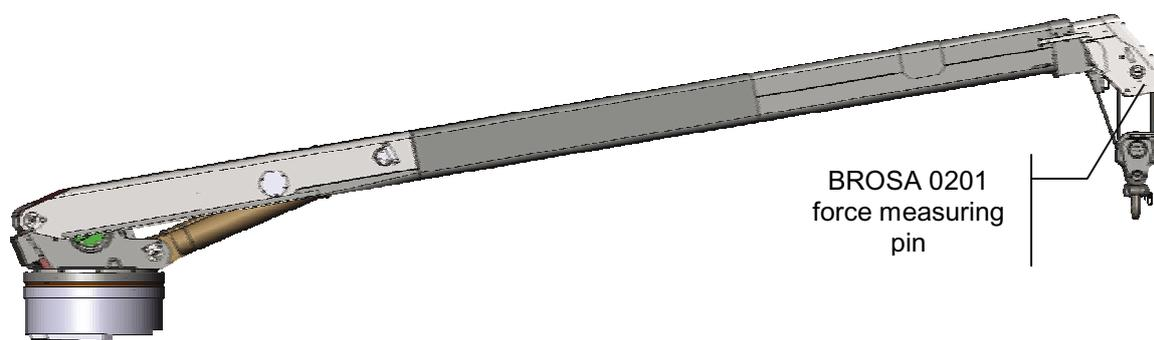
**Fig. 1. Location of the transducer on the Z10 crane**
