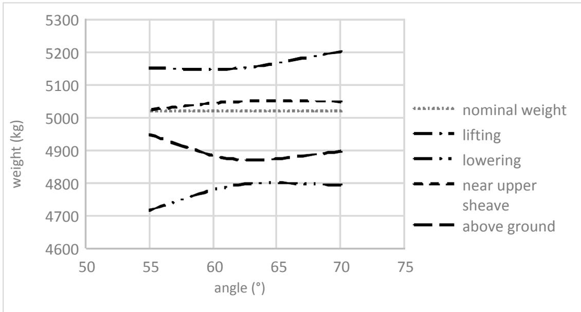
**Fig 4. Differences in indications for a 5,020 kg load**
