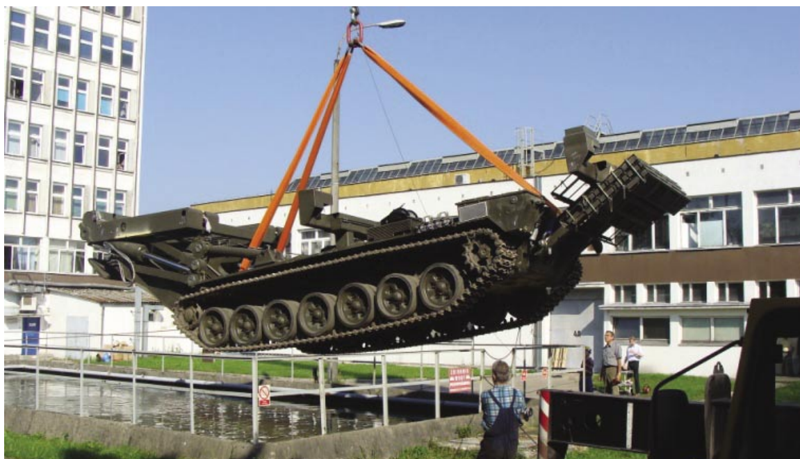
Fig. 4. Determination of chassis displacement force [2]
