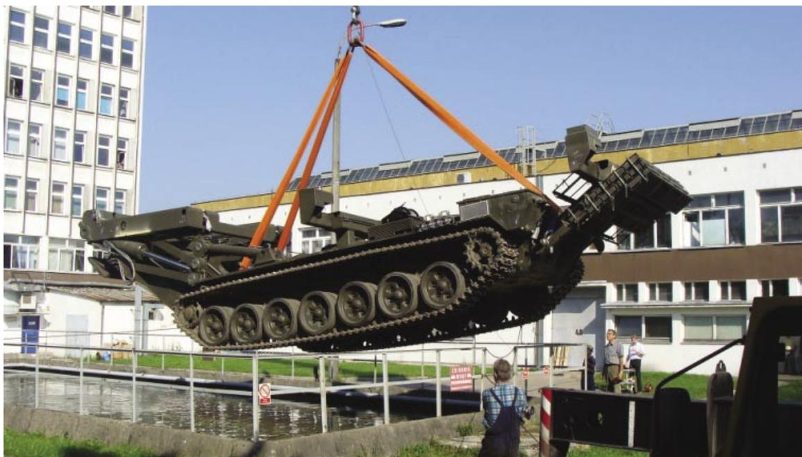
**Fig. 4. Determination of chassis displacement force [2]**
