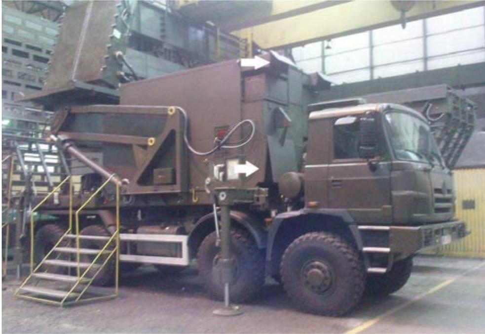
**Fig. 1. JBR-15M radar station with indicated ventilation system inlets**
