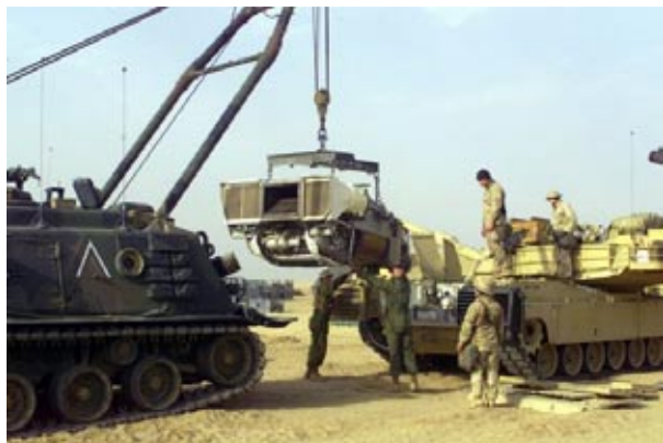
Fig. 1. Replacement of the drive unit in an ABRAMS vehicle
