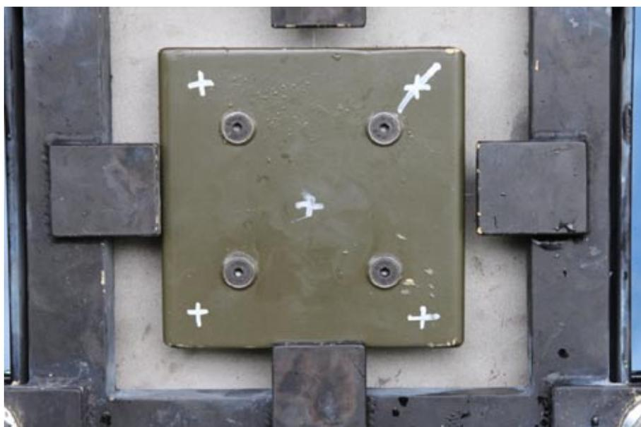
**Fig. 4. Sample piece of armour installed at the test stand**
